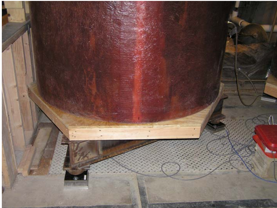
Figure 3.1. The support system of the M 2 manhole
