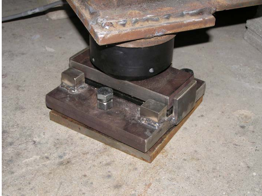
Figure 3.2. Load cell mounted on a transfer plate
