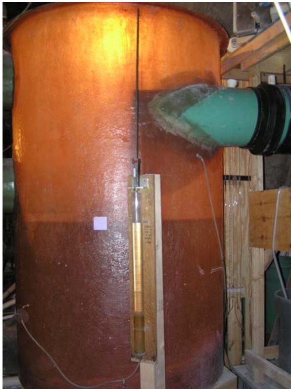
Figure 3.5. Point gage measurement of water surface elevation in the primary manhole
