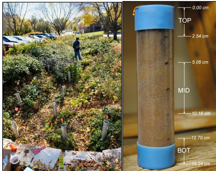
Figure 5. Running infiltration tests on a bioretention practice to map its spatial capability to infiltrate water (Left Picture) and soil core collected to determine the depth of higher metals concentration (Right Picture)
