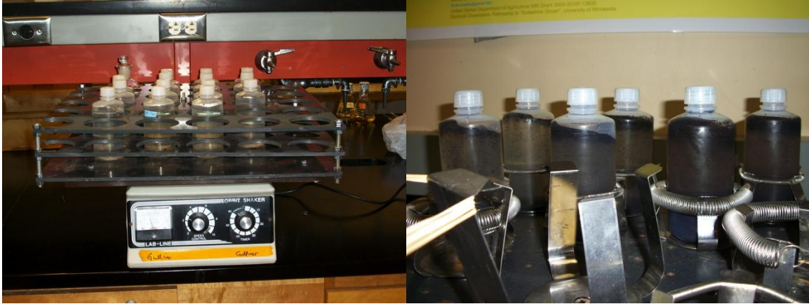
Figure 24. Shaker table and bottles used in batch study (left) and close-up of bottles on table (right).
