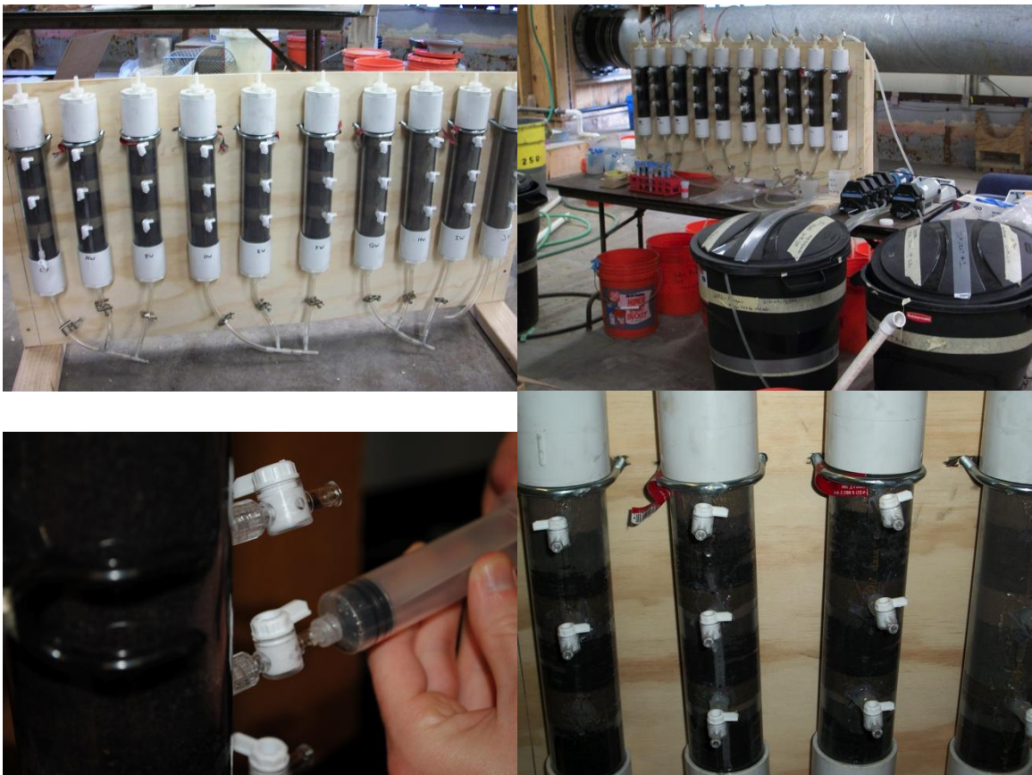
Figure 30. Clockwise from top left: 10 columns attached to support structure, Column experiment setup including influent reservoirs and pumps, Close-up of water flowing up through individual columns, Close-up of sampling procedure.
