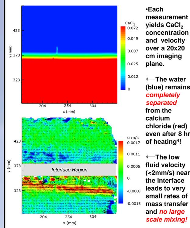
•Each measurement yields  $\text{CaCl}_2$  concentration and velocity over a  $20 \times 20$  cm imaging plane.
