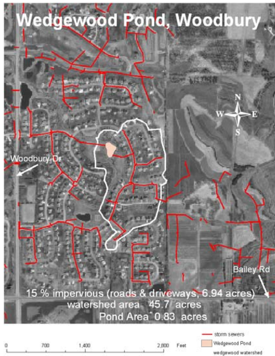
Figures 5.7.7 - 5.7.8 GIS images of stormsewer (left) and drainage area (right) near Wedgewood Pond.
