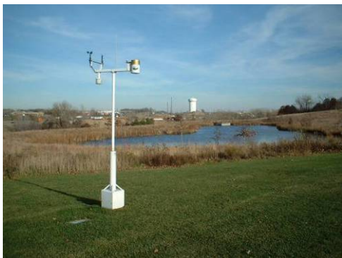
Figure 6.2.3 On-site weather station at State Farm Headquarters.
