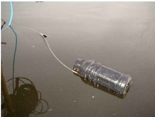
Figure 6.2.2 Thermistor, attached to underside of floating body, recording surface temperature.
