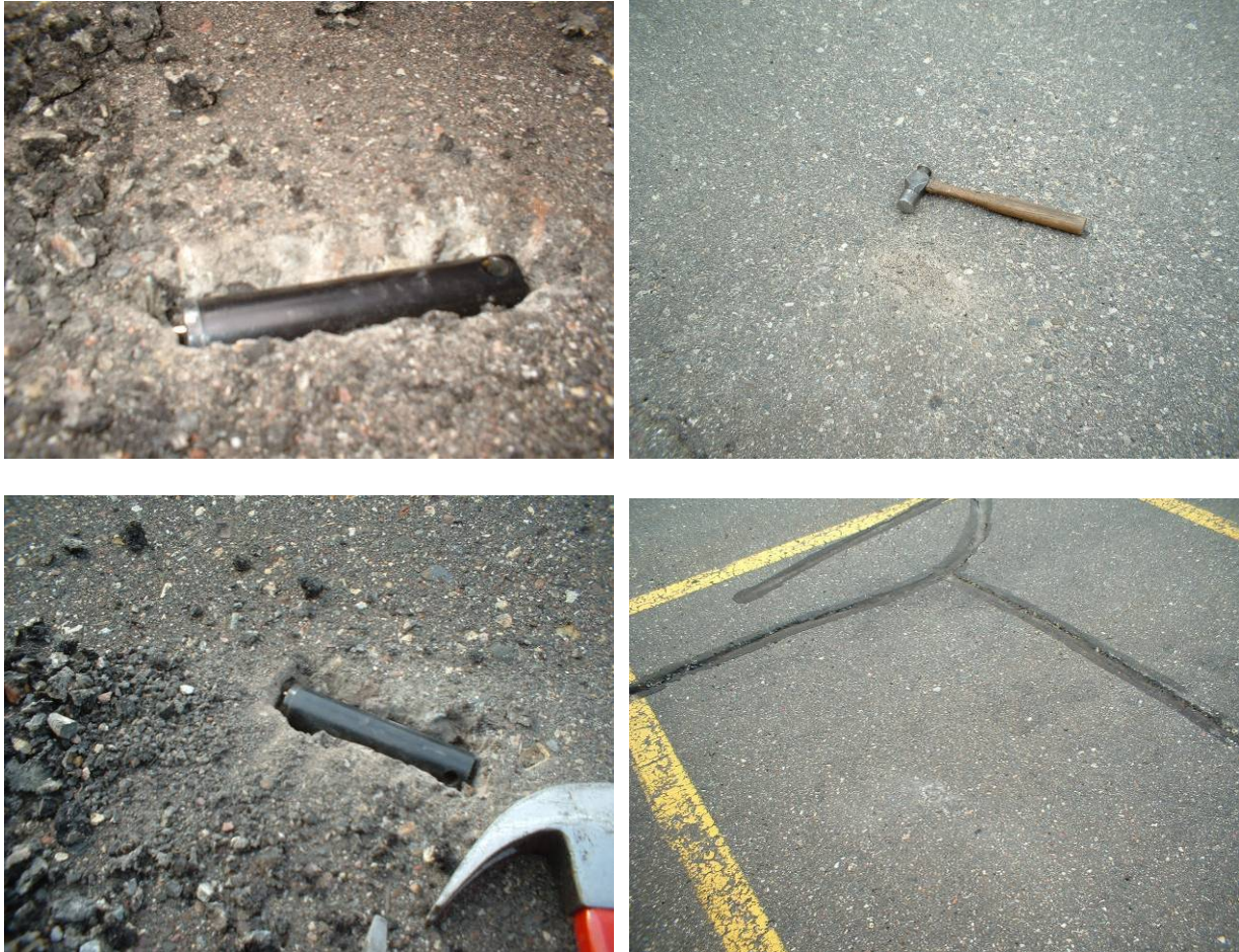
Figures 6.2.10 – 6.2.13 Vemco temperature loggers buried in upper and lower parking lot pavements.
