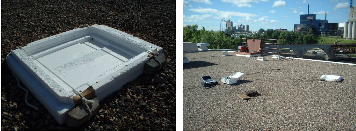
Figures 6.6.1 - 6.6.2 Rainfall temperature was measured by a thermistor placed in the drain hole of a styrofoam rainwater collector (left panel) on the roof of the St. Anthony Falls Laboratory (SAFL) at the University of Minnesota in Minneapolis (right panel).
