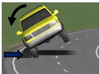
Roll from lateral inputs
