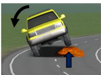
Rollover from vertical inputs
