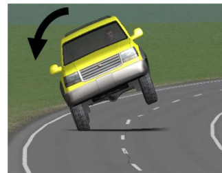
b) Un-Tripped Rollover
