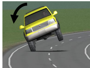
b) Un-tripped Rollover
