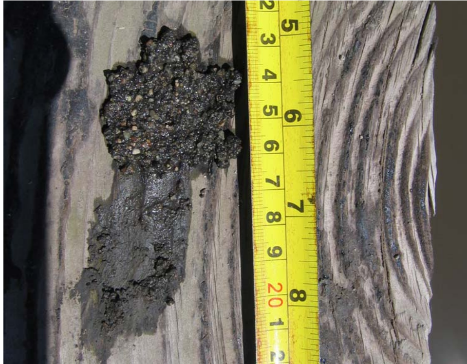
Figure 3. Pellets formed from fine silt and clay particles sampled from the bed of the South Branch Buffalo River.
