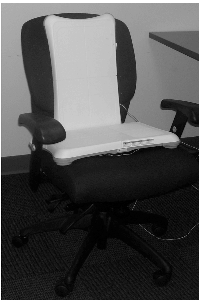
Figure 5. Gross Body Movement Measurement Device with Wii Fit Boards
