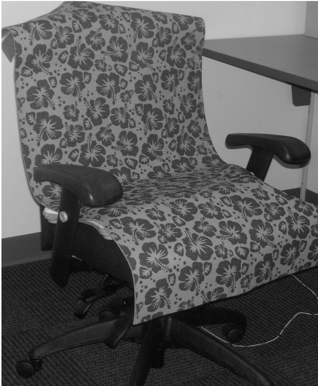
Figure 6. Gross Body Movement Measurement Device for Participant Use
