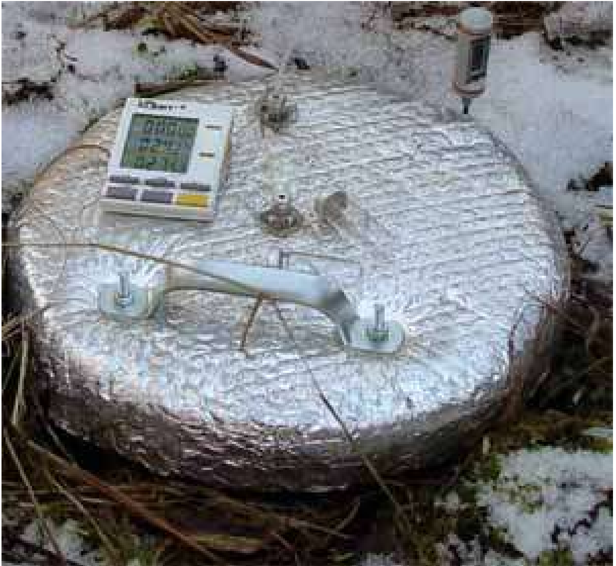
Figure 1-3. This is the top view of the two part static trace gas sampling chamber. The base of the chamber was a steel collar inserted partway into the ground. The insulated top fit over the base with a gas-tight seal. The top was fitted with a vent tube (seen here as plastic for pre-sampling and later replaced with stainless steel for sampling) and a sampling port with self-closing septa, which was replaced every third week.
