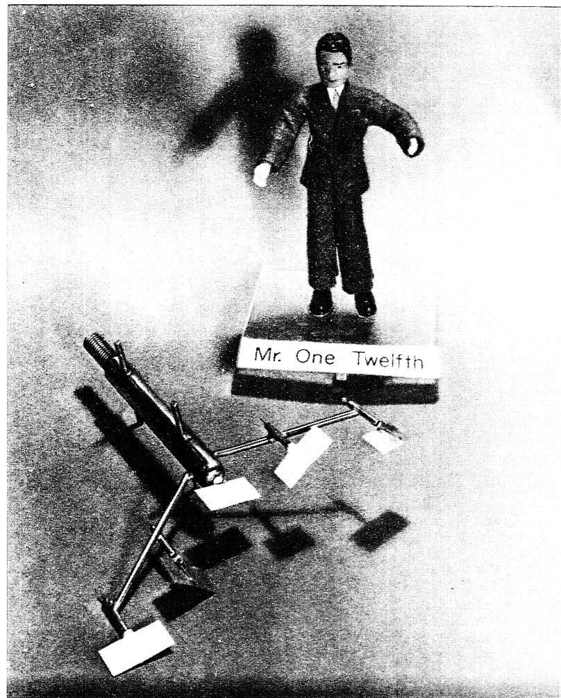
Fig. 19 - The Rotatable Vortex Sensor Assembly.
