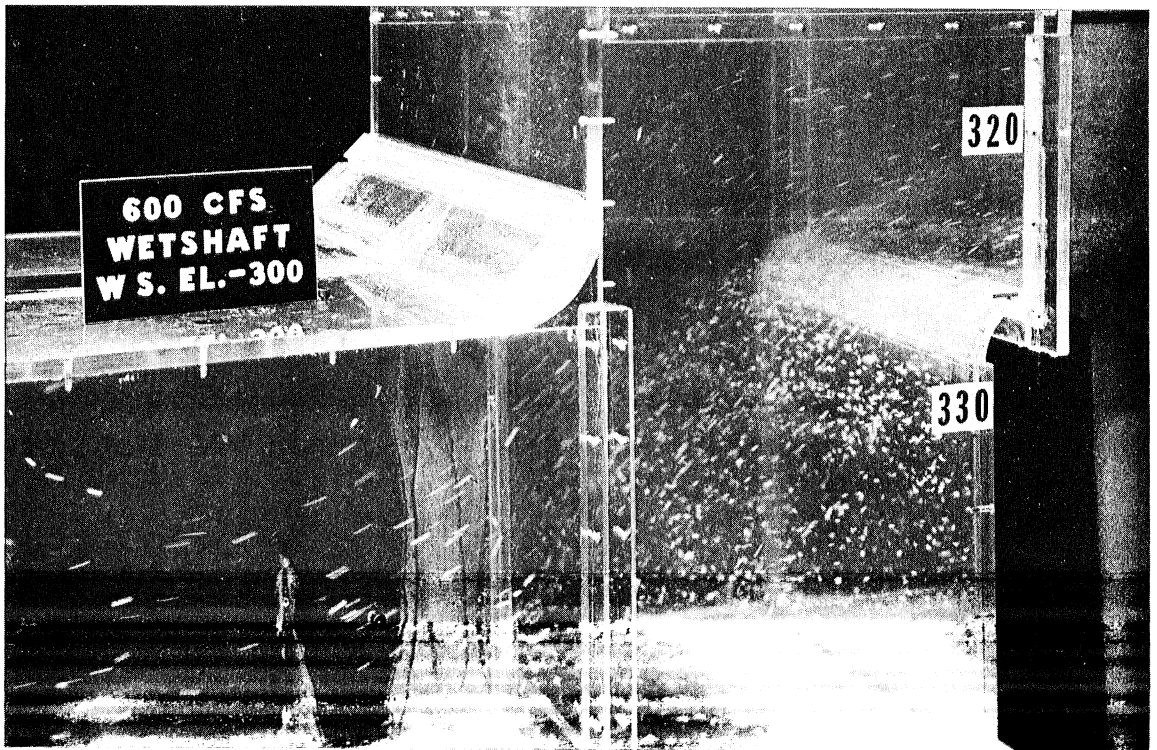
Fig. 16 - Detail of Flow Visualization at High Stage Showing Large Separation Region in Drop Structure and High Velocities near Crown of Divided Duct.
