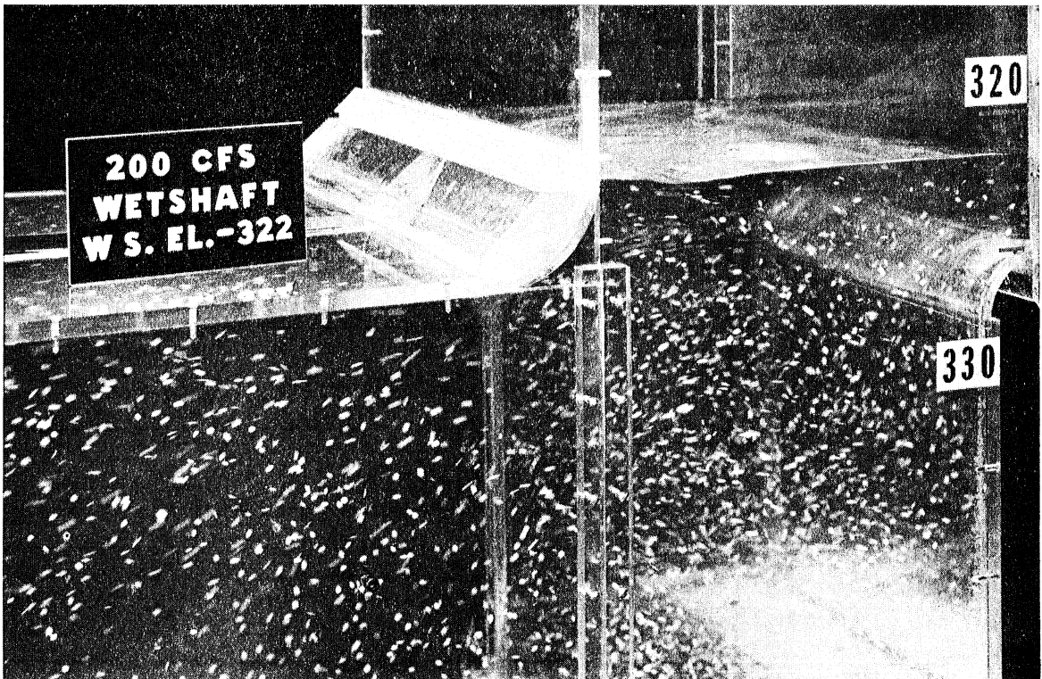
Fig. 20 - Flow Visualization of Transition from Drop Structure to Divided Duct at Low Stage. Design B.
