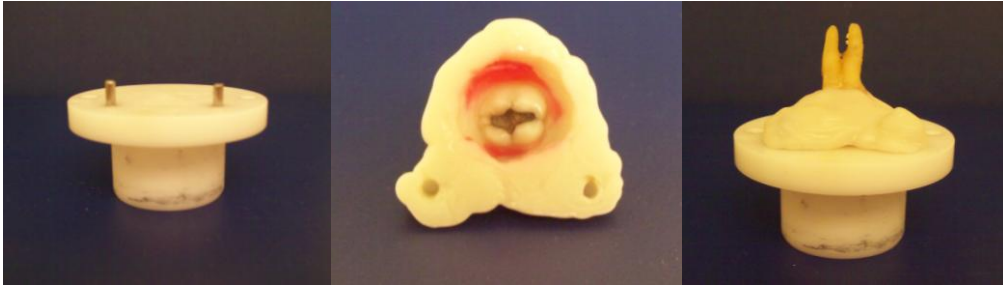
Figure 2: Mounting jig, access to the occlusal aspect of sample, and the sample mounted in the jig.
