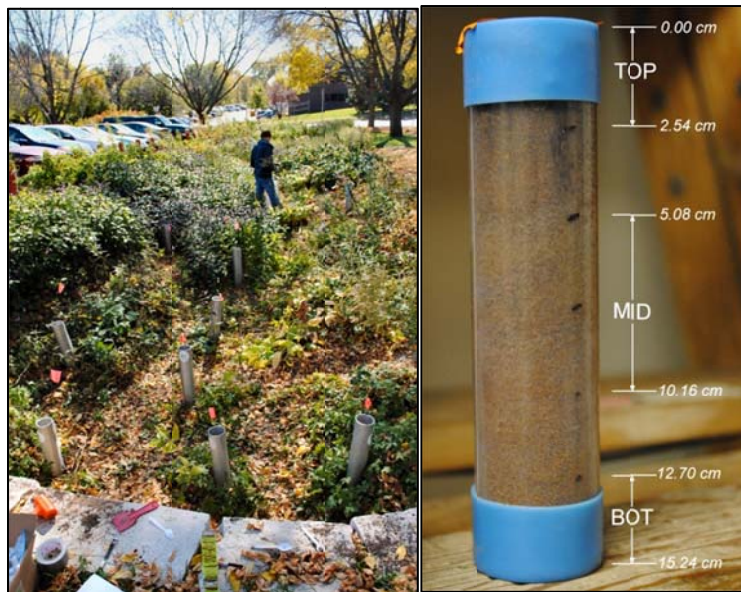
Figure 2. Running infiltration tests on a bioretention practice to map its spatial capability to infiltrate water (Left Picture) and soil core collected to determine the depth of higher metals concentration (Right Picture)
