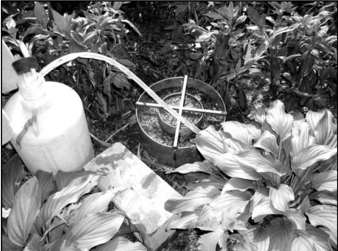
Figure F.4. Photograph of double ring infiltrometer with Mariotte system.
