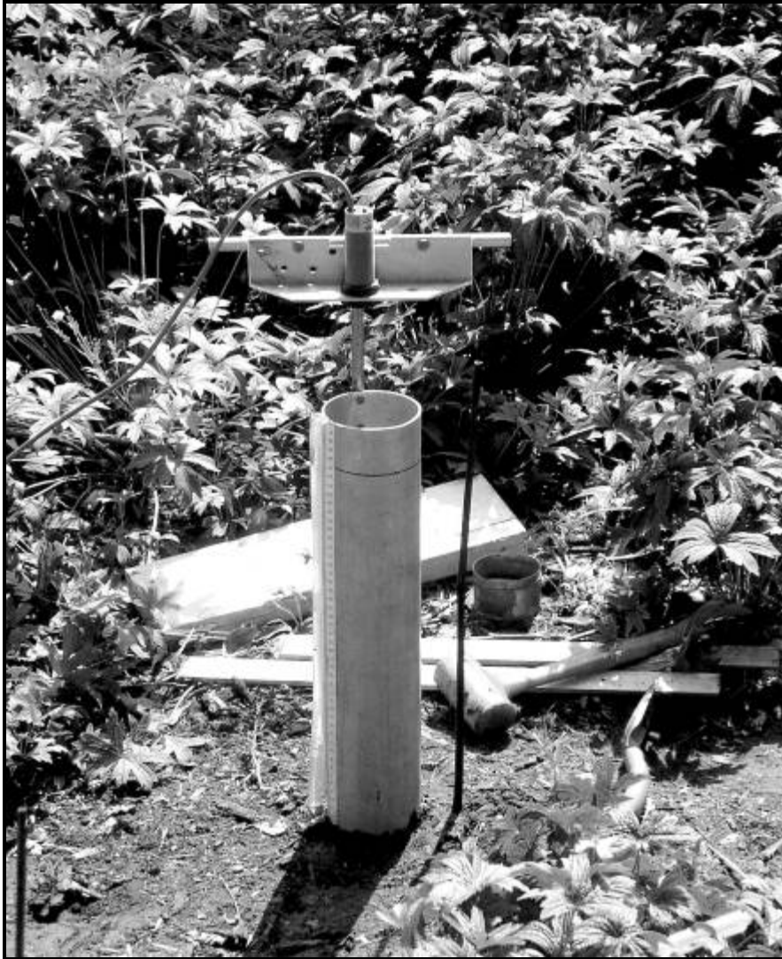
Figure F.5. Modified Philip-Dunne infiltrometer with ultrasonic sensor.
