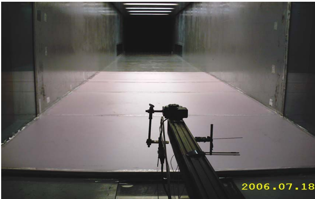
Figure 2.2: Setting up the foam board model in the tunnel
