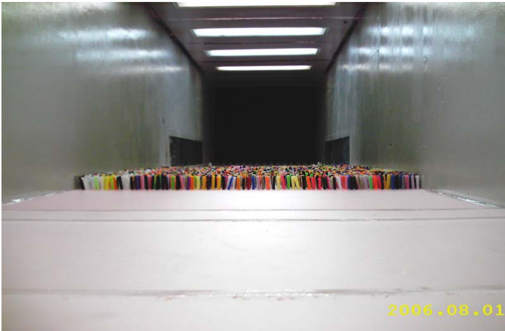
Figure 2.3 Wind tunnel test section with canopy made of pipe cleaners
