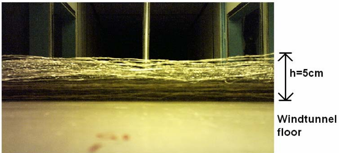
Figure 2.2: Canopy represented by chicken wire mesh, 98% porosity, 5cm height
