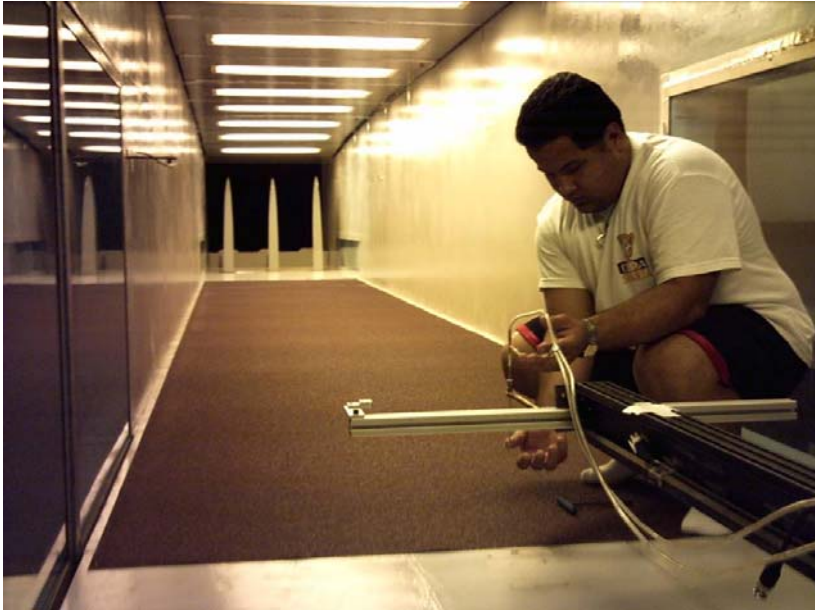
Figure 2.1. Test section of the St. Anthony Falls Laboratory wind tunnel
