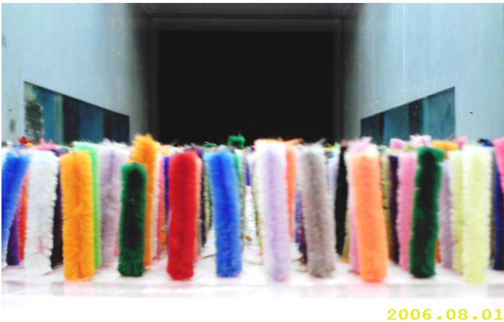
Figure 2.4: Close-up view of canopy made of pipe cleaners
