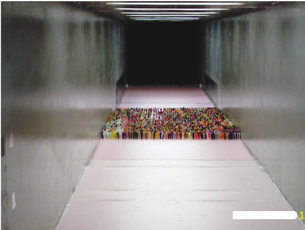
Figure 2.2 Wind tunnel test section with canopy made of pipe cleaners
