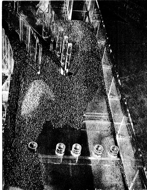
Fig. III-4 - Bed Deposits formed at 620 mgd with Grit Type 1 after Installation of Baffle Blocks (Series III)
