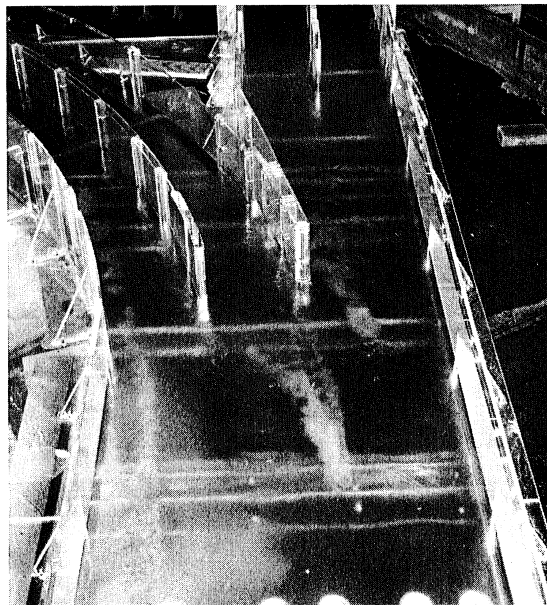
Fig. P-2 - Bottom Flow Pattern past Piers at 273 mgd as made visible by Sediment Streaks
