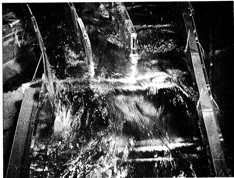
Fig. I-5 - Overhead View of Flow into the Diversion at 620 mgd (Series I)
