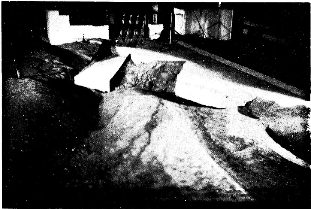
Photo 16 - Scouring Immediately Downstream of Concrete Exit Channel after 90 minutes of discharge at 5700 cms
