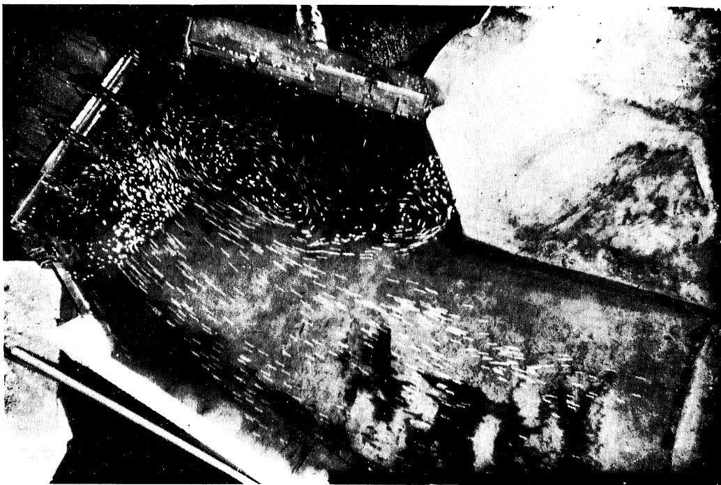
Photo 4 - Surface Flow Pattern in Approach Channel, Q = 3000 cms
