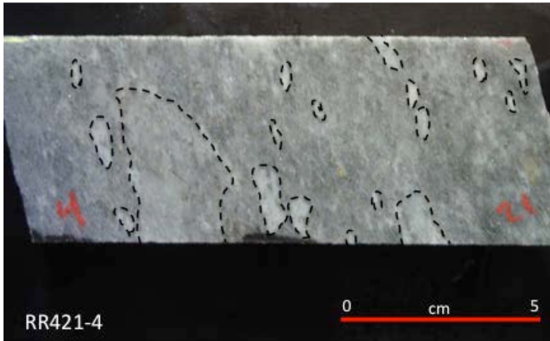
Figure 19. Drill core sample of monomictic lapilli tuff. The clasts are dacitic in composition and elongated parallel to the foliation. The majority of the clasts are <1-2 cm with rare clasts up to 4 cm long.
