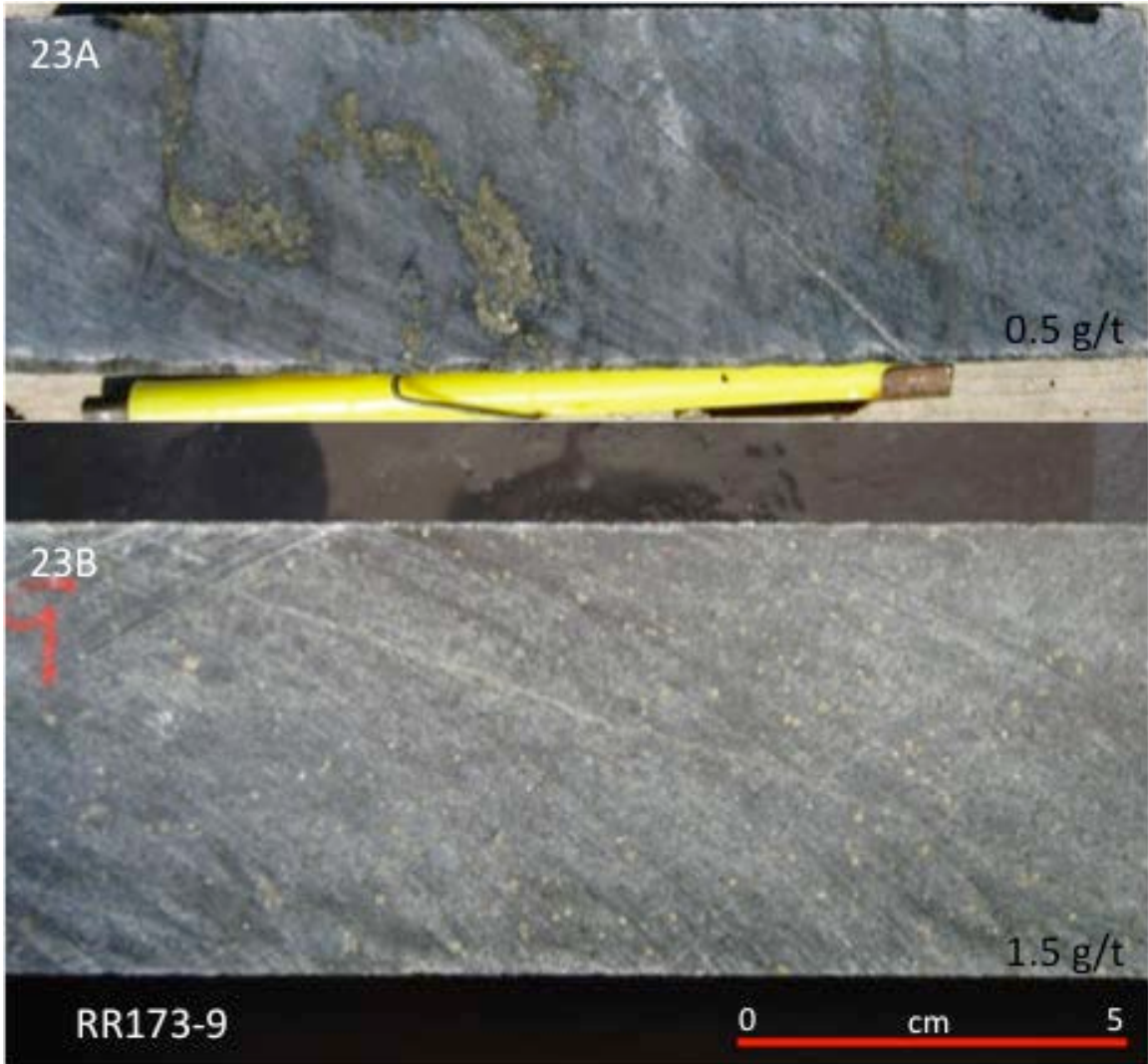
Figure 23. Two styles of low grade gold mineralization at the RRGP. Sample in Fig. 23A is characterized by tightly folded pyrite stringer veins and disseminated gold in moderately altered rocks (Fig. 23A is modified from Hrabí and Vos, 2010). Sample RR173-9 in Fig. 23B is dominated by gold hosted in open space filling pyrite associated with quartz filled amygdules.
