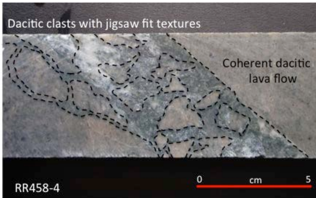
Figure 18. Drill core sample of hyaloclastite. The clasts with curvilinear and jigsaw fit margins are identical in composition to the surrounding dacitic lava flows. Secondary minerals have recrystallized the interstitial tuff between the individual clasts.
