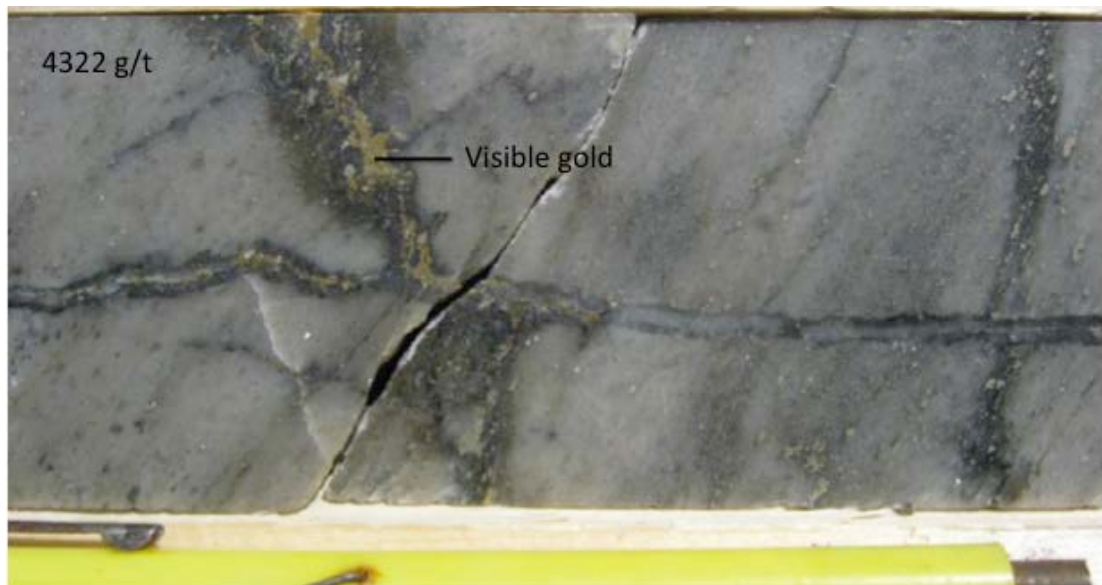
Figure 25- High grade gold mineralization in which visible gold is associated with chalcopyrite and quartz in stringers. Modified from Hrabí and Vos (2010).
