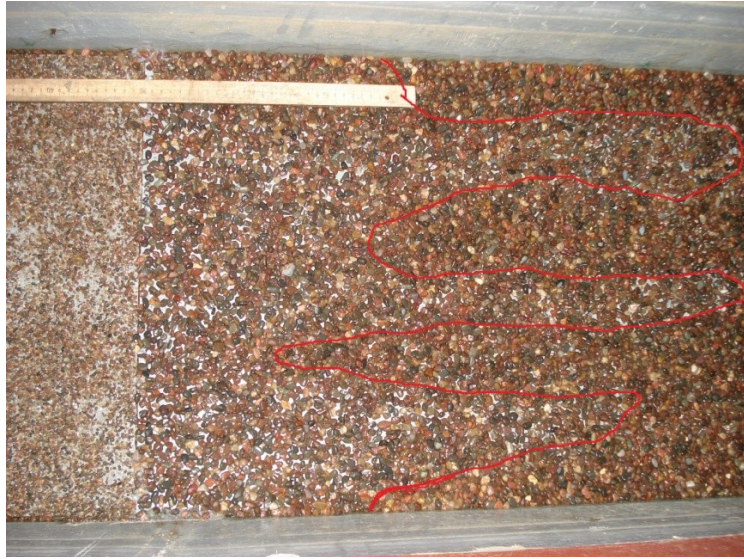
Figure 3.22. Photograph of the streaks of gravel upstream of the fixed bed R-S transition as mentioned in the text.
