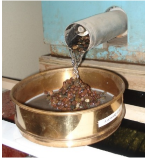
Figure 2.8. Shown in the photograph is the setup to collect a minute long sample to determine the sediment feed rate.
