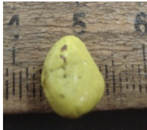
Figure 2.3. Photograph of one of the tracer gravel particles used for the experiments. The reference dimensions in the picture are cm.
