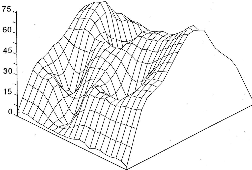
Fig. 9 The error standard deviation surface for existing monitoring network.
