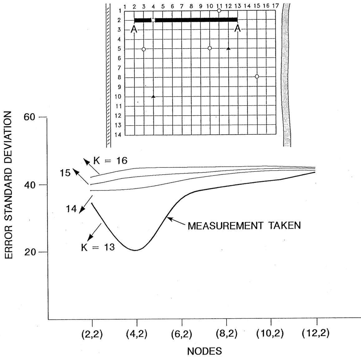
Fig. 10 The error standard deviation for cross section A-A.
