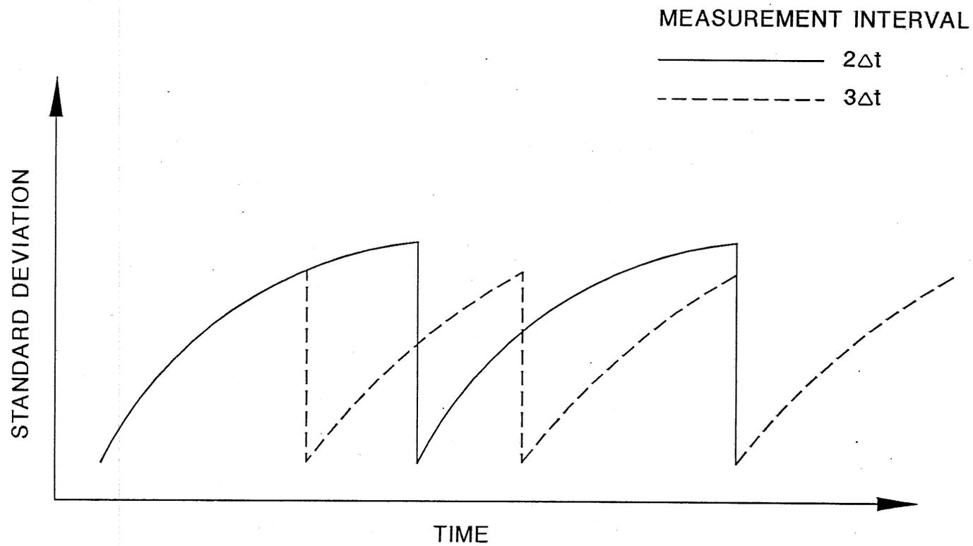
Fig. 6 Effect on changing measurement frequency on the estimation error variance.
