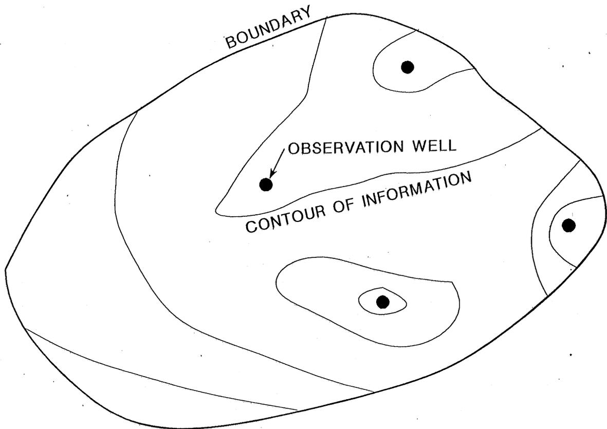
Fig. 3 Typical infograph for piezometric levels of a hypothetical aquifer.
