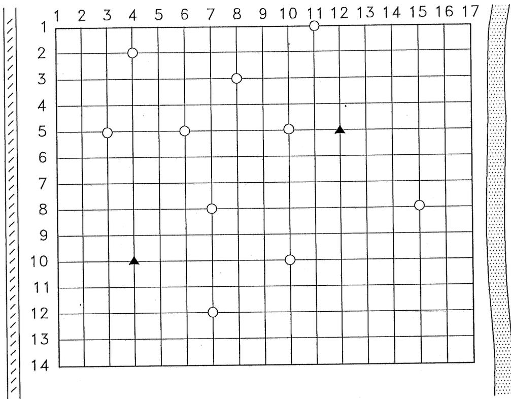
Fig. 17 The alternative with 12 monitoring wells.
