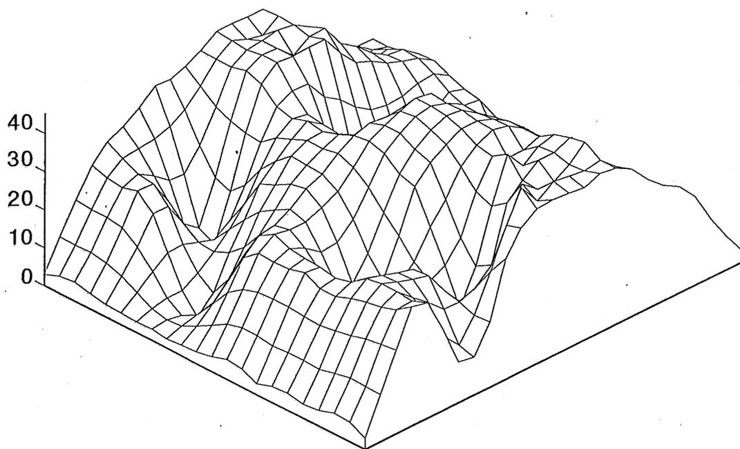
Fig. 23 The error standard deviation surface for the optimal network design.
