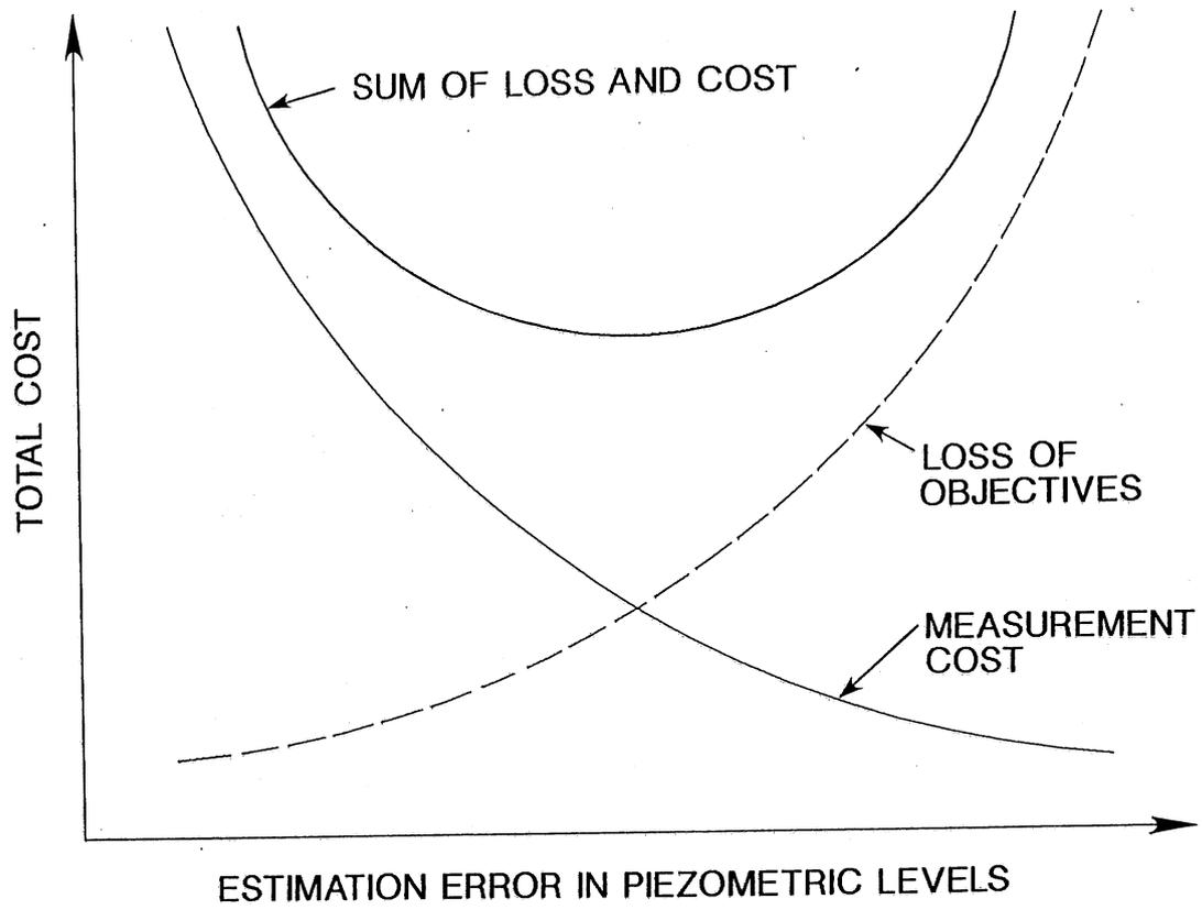
Fig. 2 Relationship between estimation error and monitoring cost.
