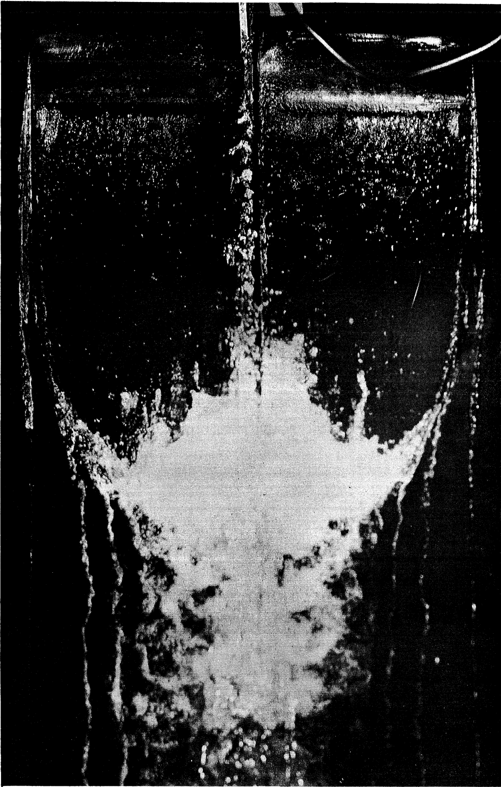
Fig. 8 - Multiple Pairs of Trailing Vortices on Cavity for Aspect Ratio 6 Flat Plate, \alpha = 10^\circ , f = 1 chord, \sigma = 0.08
