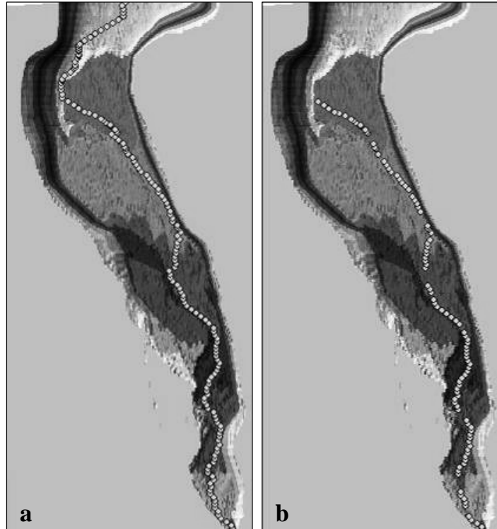
Figure 6.8. Thalweg extraction. (a) Run 2xR thalweg after 2,550 minutes as extracted by the thalweg-seeking algorithm. In sections its points change direction more suddenly than those of a real thalweg. (b) The same thalweg after these points have been manually removed.
