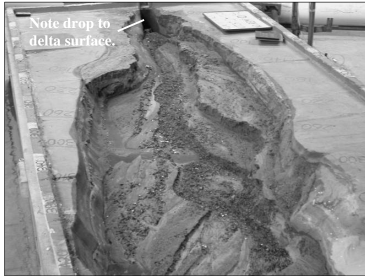
Figure 8.1. View looking upstream towards the end of run 3xC. Note the drop between the mouth of the delivery channel and the delta surface at the top of the photograph. Photograph courtesy of Corey Markfort.
