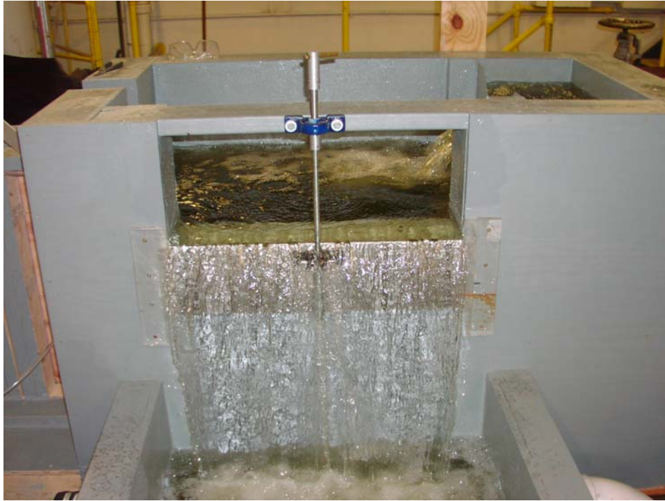
Figure 4. The side weir in the head tank to control the headwater.
