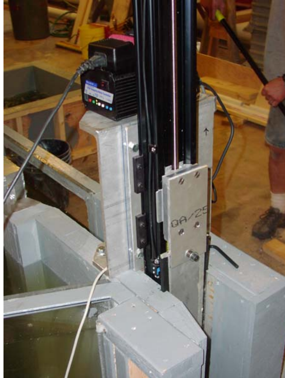
Figure 7. A Velmex slide system was utilized to automate the sluice gate opening.
