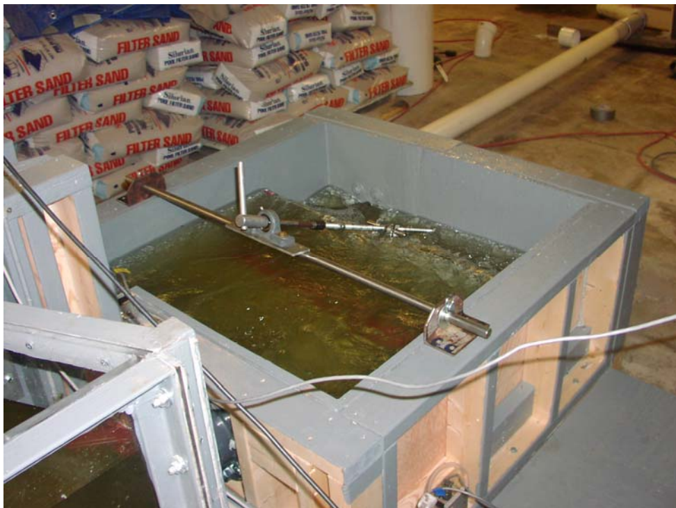
Figure 4. The side weir in the head tank to control the headwater.
