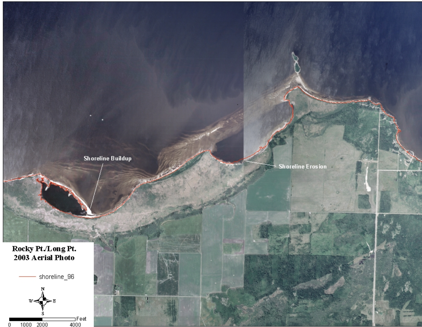
Figure 2.5. The Lake of the Woods shoreline area between Rocky Pt. and Long Pt. in 2003 and in comparison with the 1996 shoreline.
