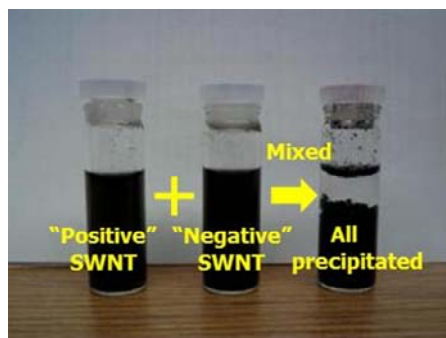
Figure 5.4: Precipitating reaction occurred by mixing two oppositely charged SWNT dispersions.
