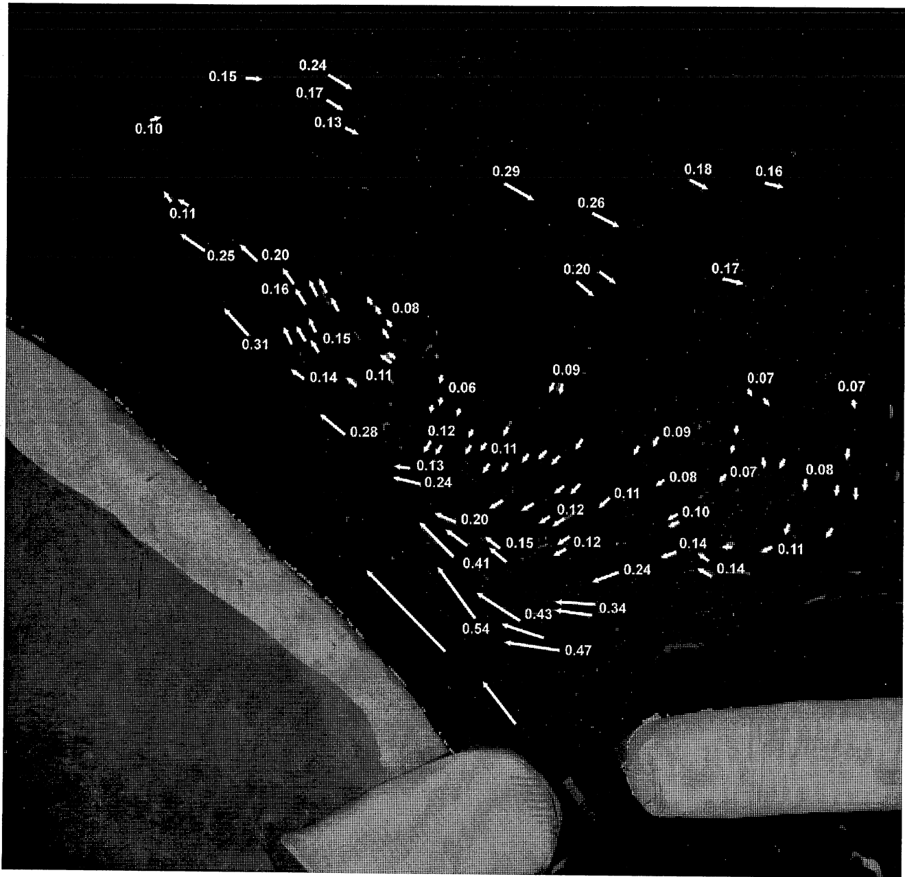
Figure 22 Surface flow velocities along the east shoreline for a flow of 25,850 cfs with the embankment in place.
