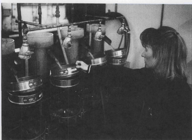
Tests for soybean cyst nematode (SCN) are performed in the nematology laboratory at the Waseca Center. Along with confirming SCN presence, the test provides an estimate of cyst nematode population densities. Cathy Johnson operates an elutriator, which washes nematode eggs from soil samples. Information on the test is available at county extension offices or toll-free from the SCN Coalition, 1-877-726-8378
