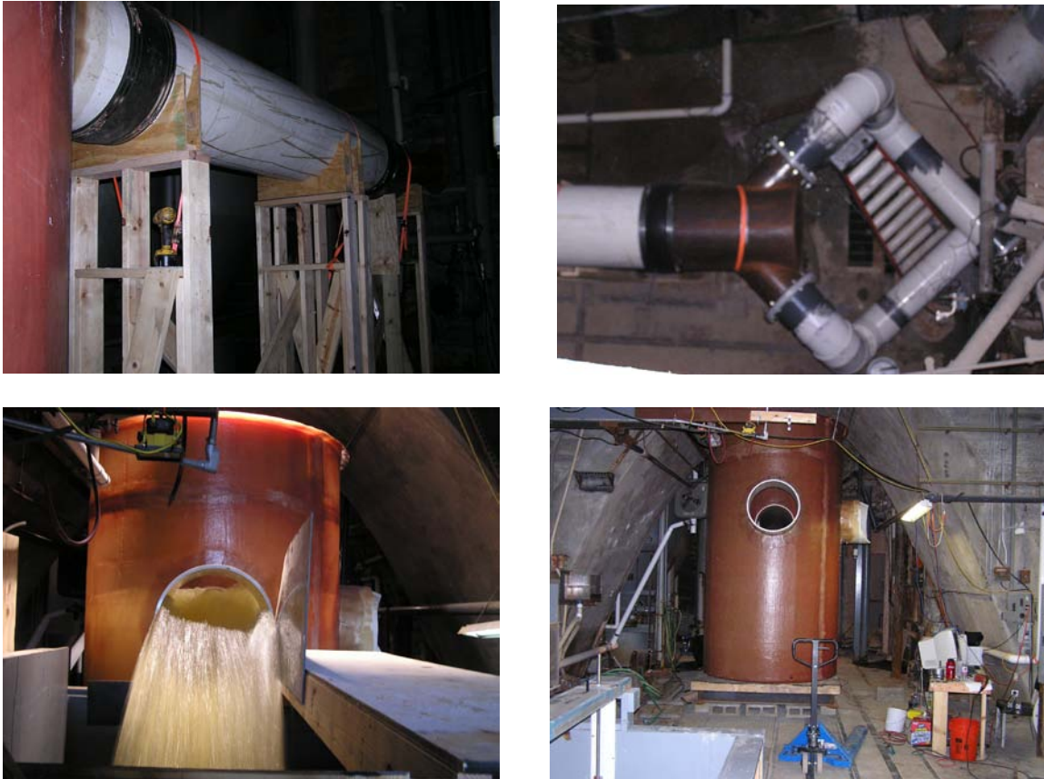
Figure A.4. 6-ft Sump Setup
