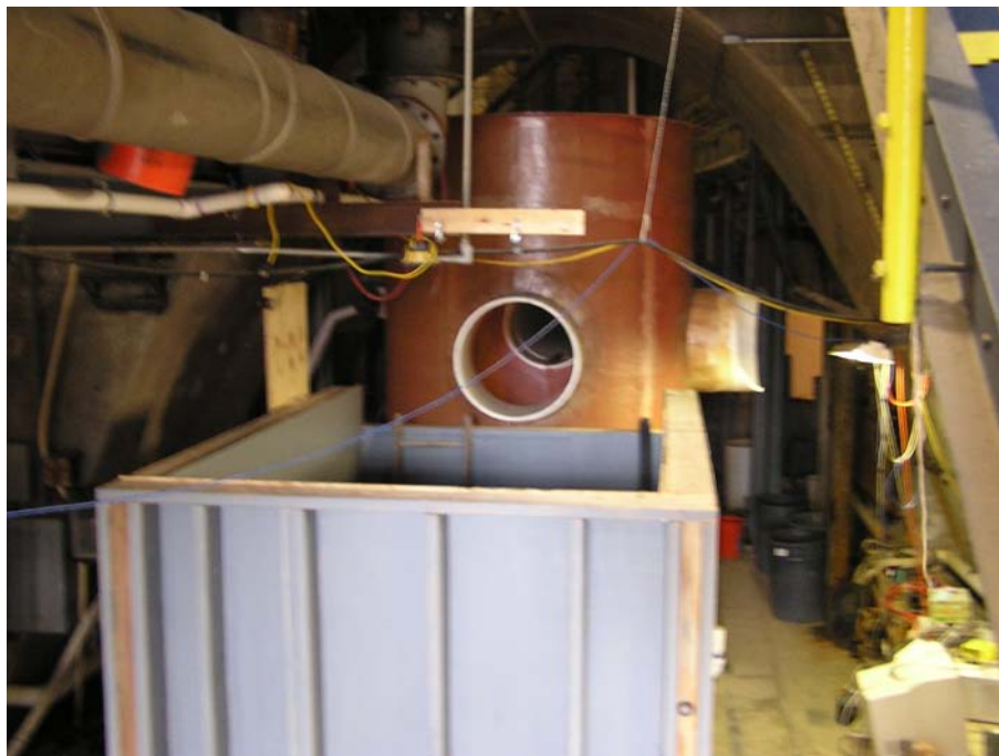
Figure 2.2. 6×6ft Sump and Tailwater Box
