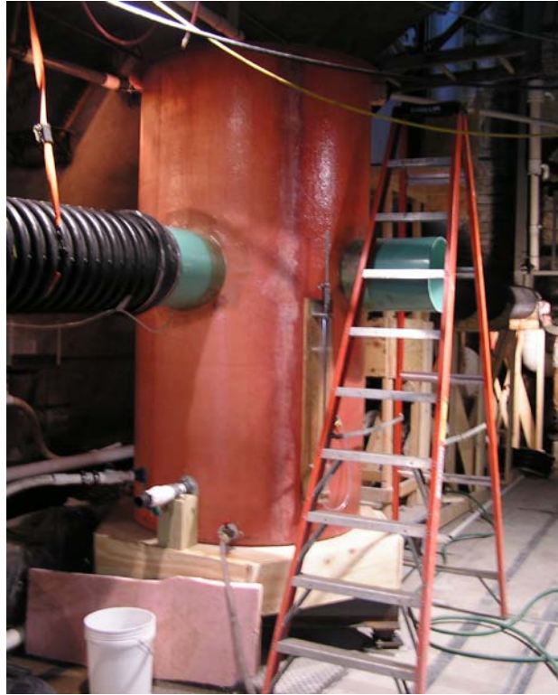
Figure 2.1. 4×4ft Sump and Test Stand
