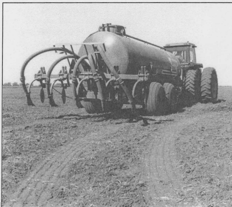
A 3,000 gallon liquid manure tank and injection system handles about half the manure generated by station livestock. Returning manure to the soil in this manner helps preserve the nutrients for use by crops.
