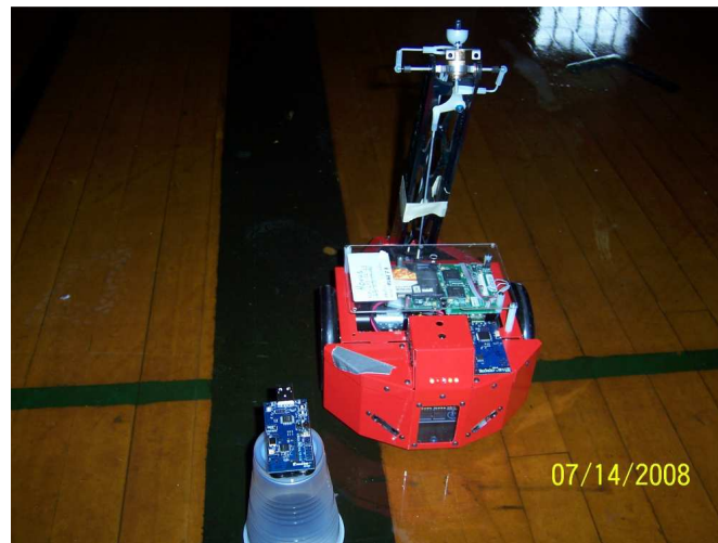
Figure 4.4: An Acroname Garcia robot visiting a sensing mote. Note the single board computer on the robot under the clear lid and the mote connected to the robot's computer.
