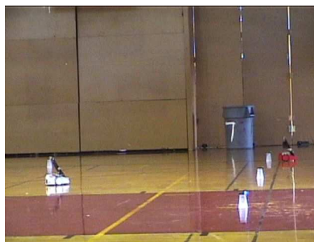
(b) A snapshot from the experiment with two mules. One mule (white robot) is following its designed path while the other mule (red robot) is downloading data from the assigned mote.
