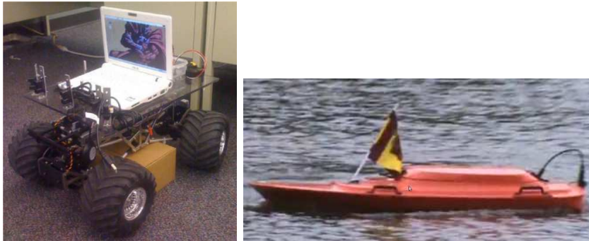
Figure 6.1: Left: Cyclops robotic platform developed for data muling. Right: Miskin robotic raft developed for tracking carp tagged with radio transmitters [4].
