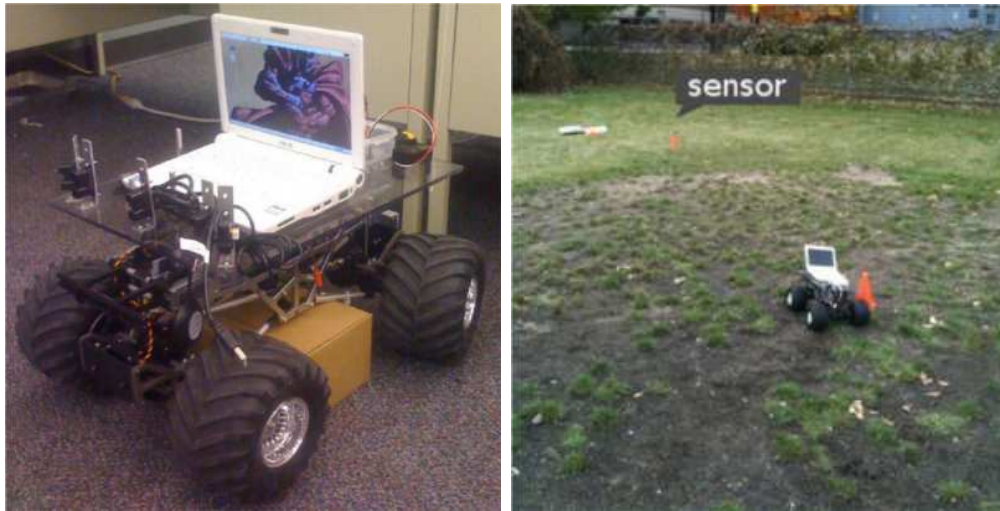
Figure 4.17: Left: Cyclops robotic platform developed for data muling. Right: A data mule system together with sensors.
