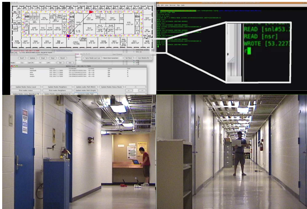
Figure 2.30: Unknown user trajectory experiment-1: This figure shows the initial locations of the mobile router network. In this experiment, the mobile router network keeps the connectivity of an adversarial user (laptop) who requests wireless connectivity and sends acknowledgment of its move in each time step. The top left figure shows the GUI, the top right figure shows the message sent from user, the bottom left figure shows the robots and base station, and the bottom right figure shows the user.
