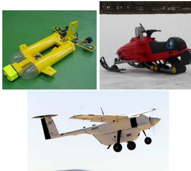
Figure 6.2: Left: Starbug robotic platform developed for data muling under water [5]. Right: Arctic Crawler robotic snowmobile developed for monitoring arctic environments [6]. Bottom: RCATS/APV-3 is a UAV developed for collecting imagery data by flying over vineyards [7].
