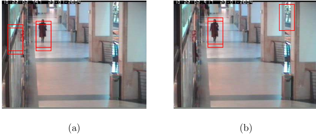
Figure 38: (a),(b) show results with using 1 and 2 background frames respectively for autonomous updates.
