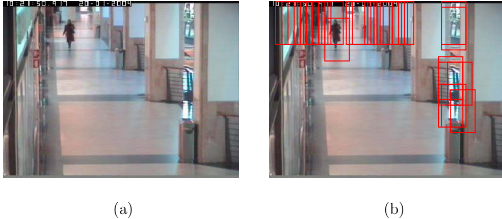
Figure 35: (a) Original frame. (b) Output of a human detector trained on the INRIA dataset.
