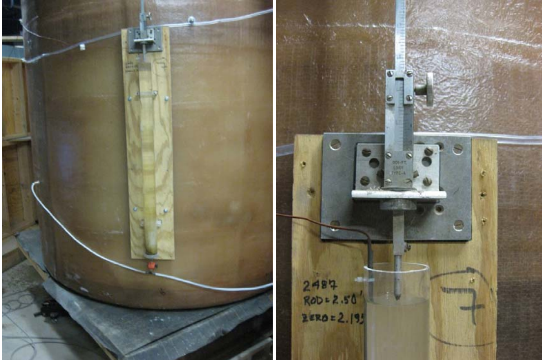
Figure C-8: Stilling basin and point gauge used for water level measurement
