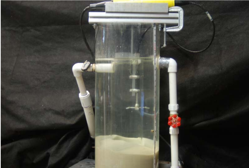
Figure 4-7: Swirl flow device scale model with ADV setup
