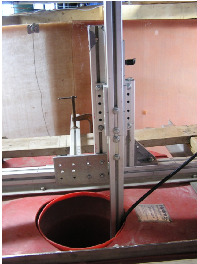
Figure 5-5: The ADV bracket installed on top of the Downstream Defender holding the ADV in the sump
