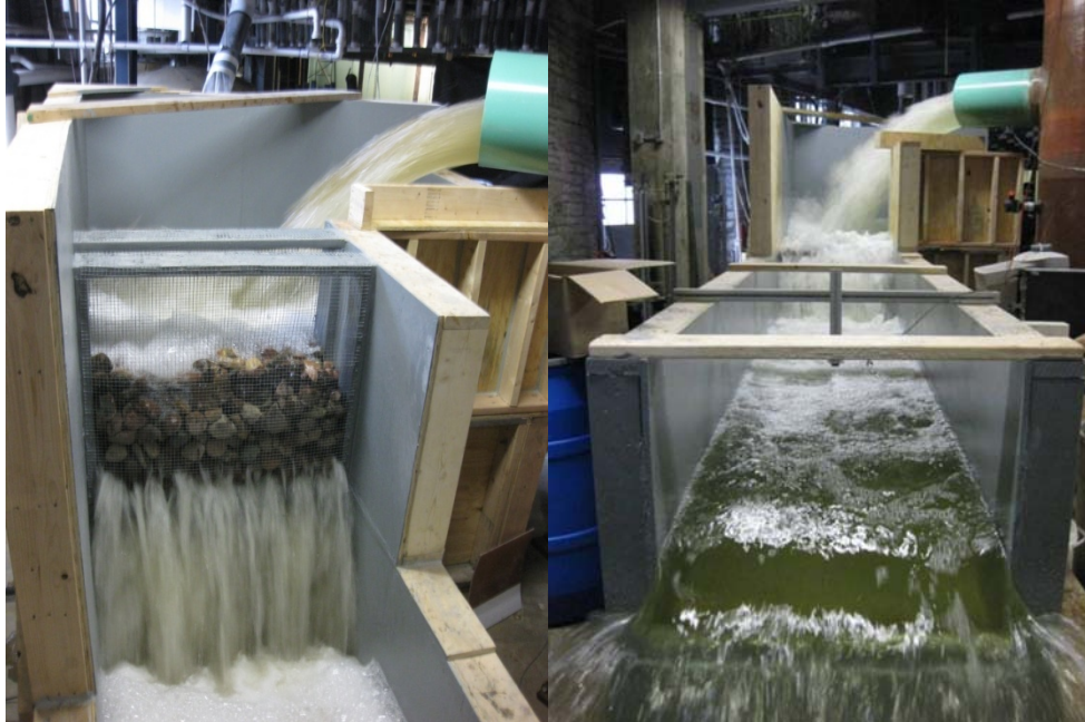
Figure A-15: Channel discharge flow measurement
