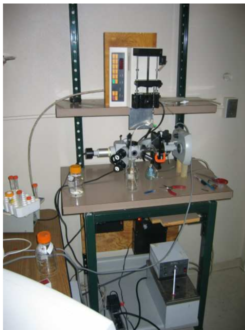
Figure II-1: Picture showing the experimental microscope based imaging system. The flow was controlled by a 0.5 \mu\text{L} syringe mounted in a syringe pump. The glass capillary was attached to the syringe pump, and the microscope was focused onto the capillary.
