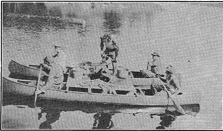
In the upper picture is shown the outfit of two canoes lashed together with a platform between, from which the depths of Minnesota lakes were dredged; below a deep-sea thermometer is shown being brought up from a hole 240 feet deep in Canadian waters of Lake Saganaga.
