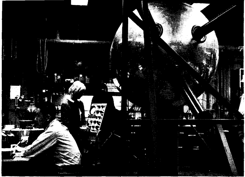
In this laboratory for reproducing the high intensity electric fields found in thunderstorms, studies are made of the role that condensing water vapor and interacting water droplets play in the generation of atmospheric electricity. Graduate students in the foreground are Mr. Chung Ching Liu and Miss Frances Anderson.
