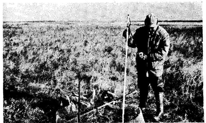
Thermocouples, which will record temperatures of the earth at four-inch intervals to a depth of five feet, are installed by John Tester.
