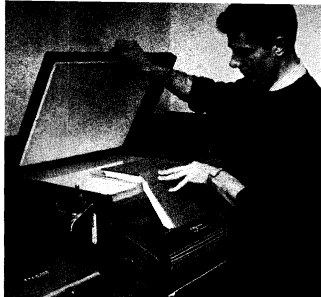
Paul D. Glass, student operator, uses the "Copease" photocopying machine to make an exact duplicate of a bound volume page. This new chemical duplicating process provides permanent, non-fading copies of any printed, typed, or hand-written material up to 14" x 17".
