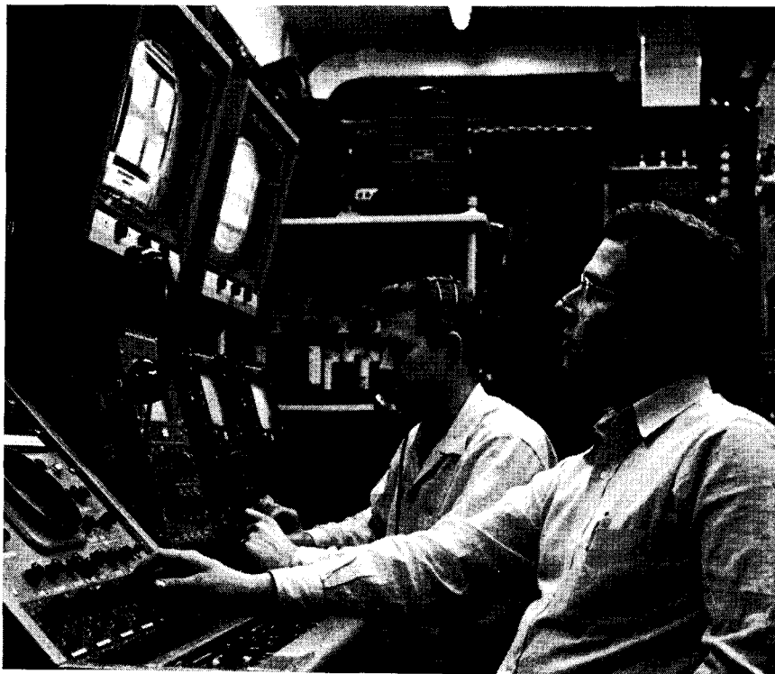
Two engineers on the Television Production Center engineering staff are shown in the control room of Studio 4. Philip Jedlicka (foreground) mans the video controls, as Everett Lindgren corrects or "shades" the camera balance of the picture.
