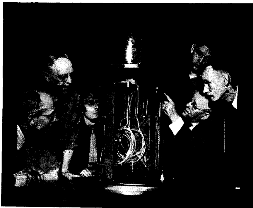
The only apparatus of its kind in the country gets the interested inspection of staff members. Showing off the new device to test insulation materials under vacuum and at low temperatures is Robert Lander, extreme left, an assistant scientist at the Station who designed the device. Looking on, left to right are C. O. Lund, mechanic; Herman Fors, senior lab attendant; Robert Rhame, machinist; Roger Erickson, senior machinist; Lauritz Clausen, machinist.
