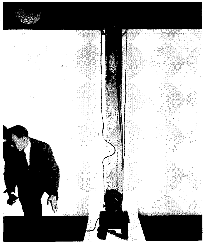
Scientist Fritjof Christensen puts Strobolight to still another use as the camera stops action in his transverse wave experiment. The belt, just struck with the hammer, is traveling at 50 feet per second.
