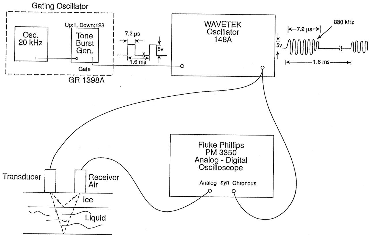
Figure 1. Laboratory pulse measuring system.
