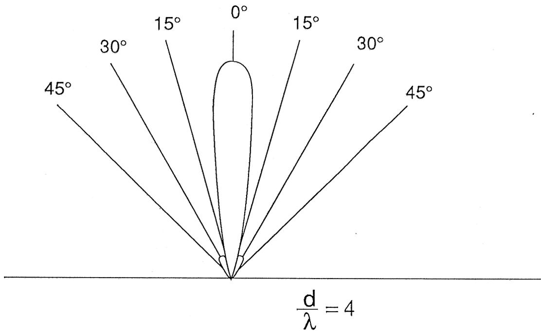
Figure 3. Theoretical transducer radiation pattern
