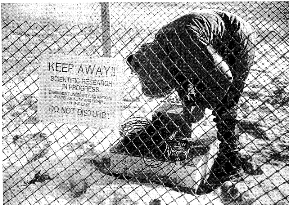
Photo 10. Datalogger platform used to monitor water temperature profiles (Feb 1990).
