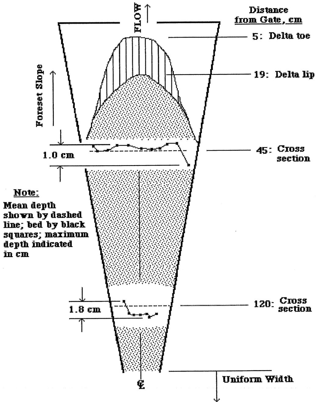
Figure A2.8 Plan view of expanding region upstream of dam for Run 17
