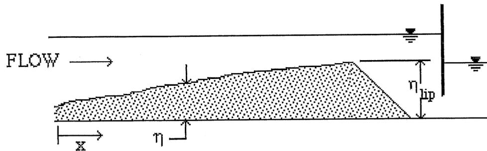
**Figure A2.14 Dimensionless longitudinal bed profile in expanding region upstream of dam for Run 19**
