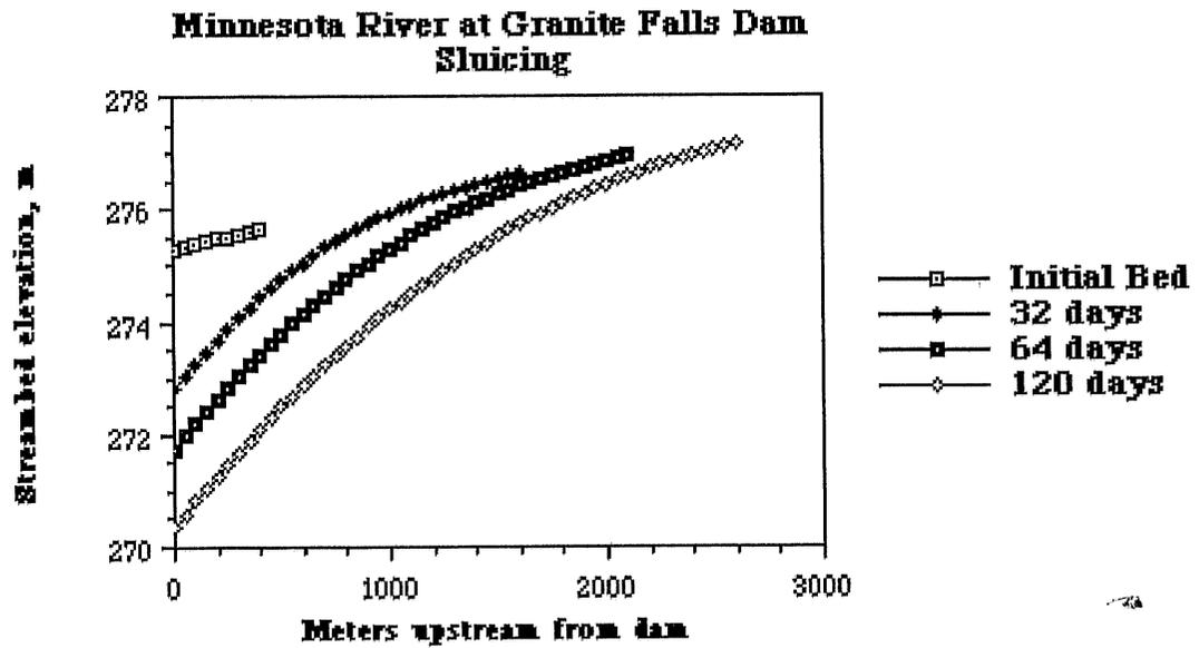
**Figure 4.16** Computed bed profiles for the first 150 days of sediment sluicing
