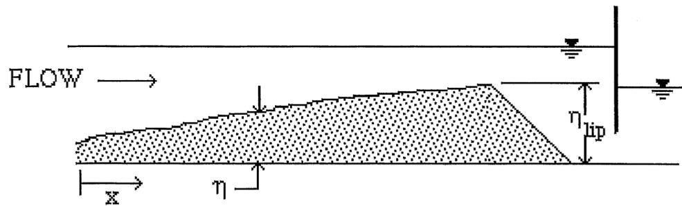
**Figure 3.9 Dimensionless longitudinal bed profile in expanding region upstream of dam for Run 19**
