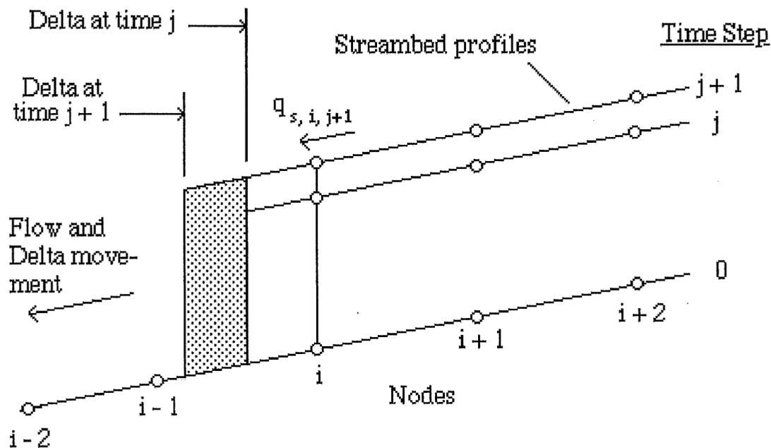
**Figure 4.2 Method of moving the shock face forward**
