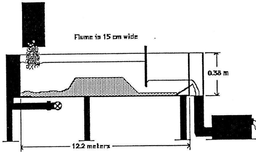
Figure 3.1 Uniform width flume (not to scale)
