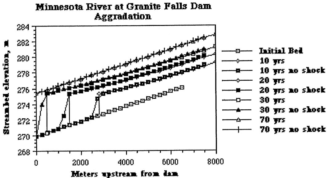
**Figure 4.14 Computed bed profiles for field case with and without the shock-fitting option**
