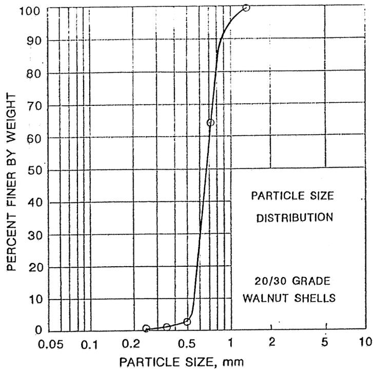
Figure 3.3 Crushed walnut shell particle size distribution
