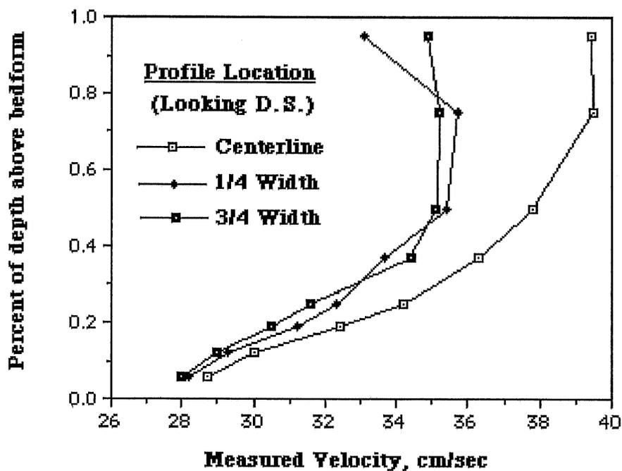
**Figure 3.7** Lateral velocity profiles for Run 17
