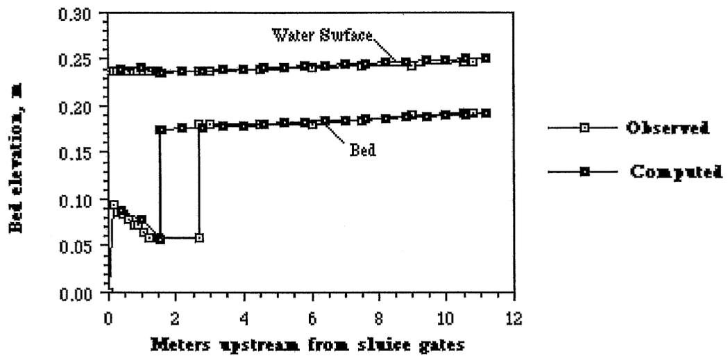
**Figure 4.6** Observed and computed bed profiles 7 hours later for Run 28
