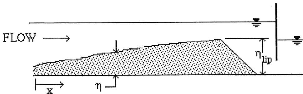
**Figure A2.12 Dimensionless longitudinal bed profile in expanding region upstream of dam for Run 17**
