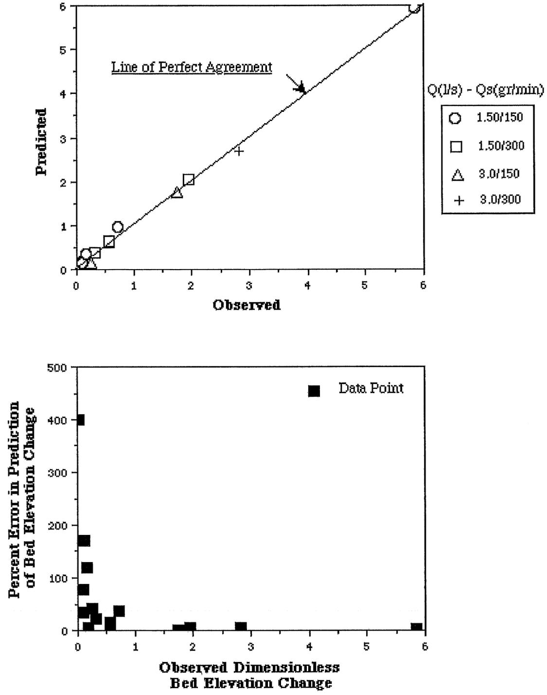
**Figure 3.14 Observed vs. predicted change in bed elevation**
