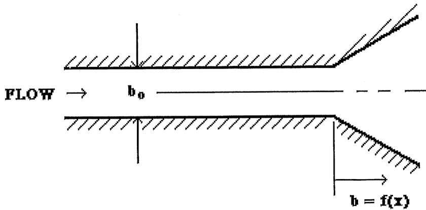
**Figure 5.2 Plan view of channel with prescribed varying width**
