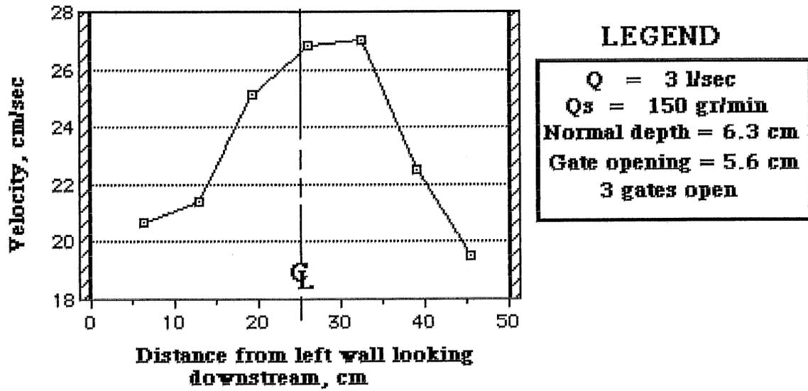
**Figure A2.16 Mean velocity at one-half depth at a location 30 cm upstream from sluice gates in diverging flume for Run 17**
