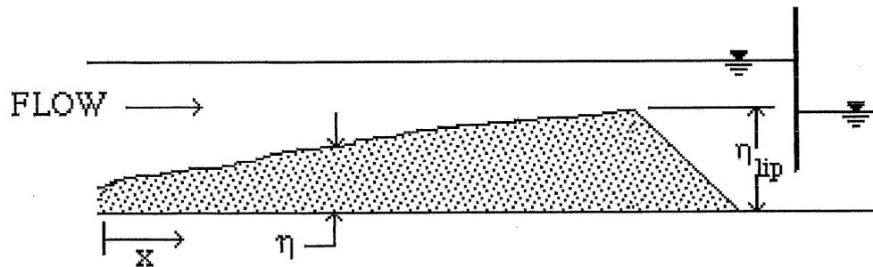
**Figure A2.15 Dimensionless longitudinal bed profile in expanding region upstream of dam for Run 20**
