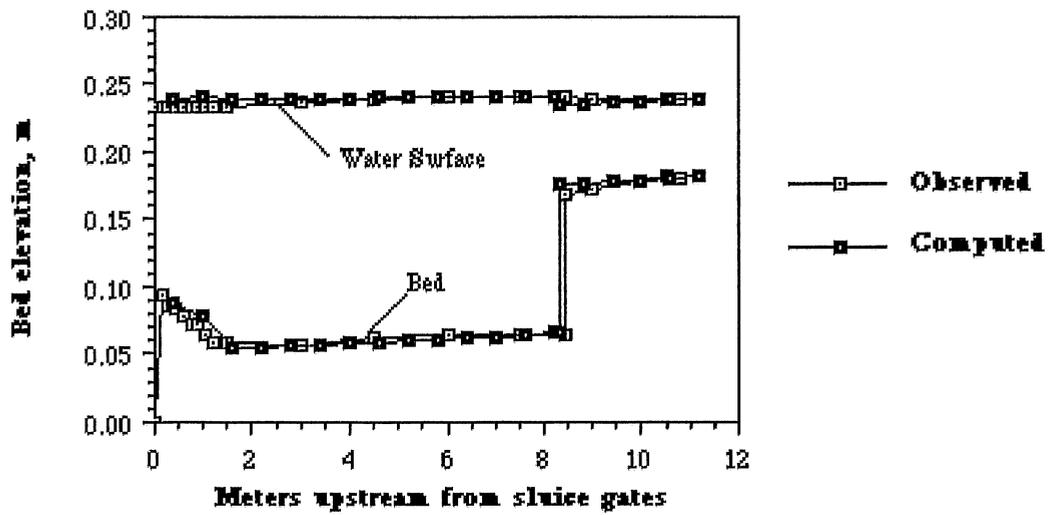
**Figure 4.5** Observed and computed bed profiles 1 hour later for Run 28
