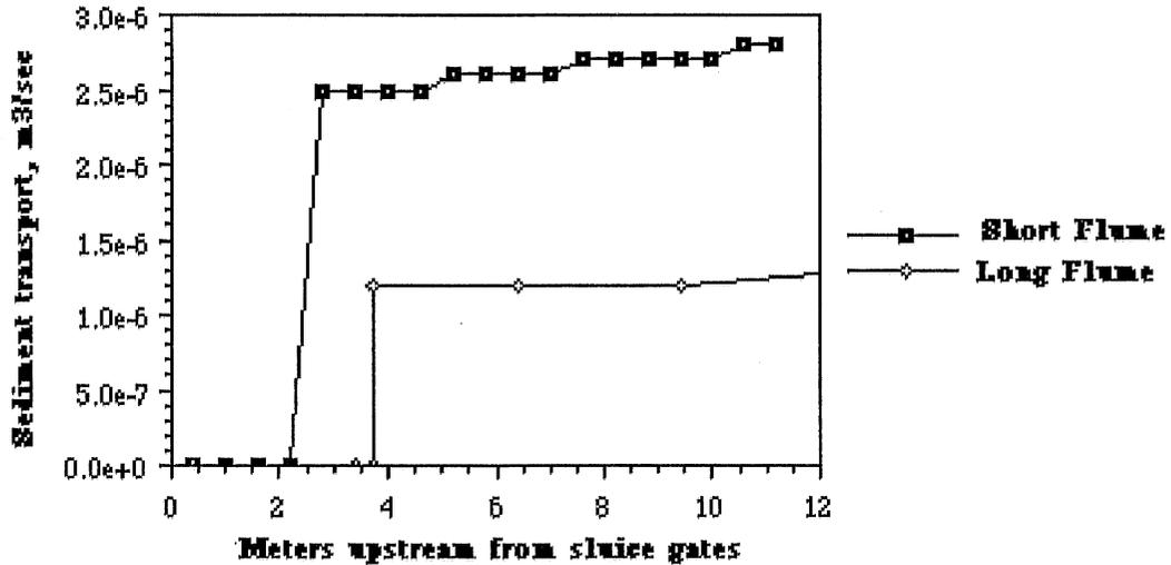
**Figure 4.8 Computed sediment transport rates for 12-meter-long and 120-meter-long backwater reaches**
