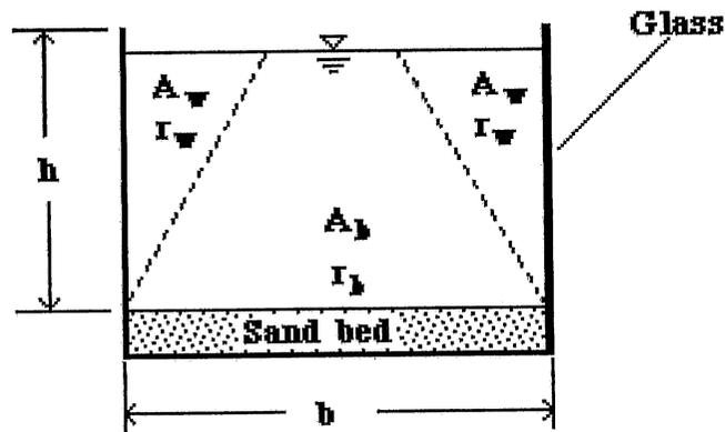
**Figure A1.1 Hypothetical division of bed and wall hydraulic parameters**
