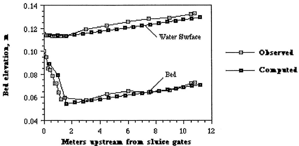
Figure 4.4 Observed and computed initial conditions for Run 28
