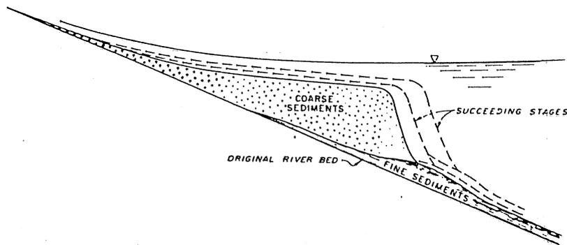
Figure 1.1 Profile of typical reservoir delta
