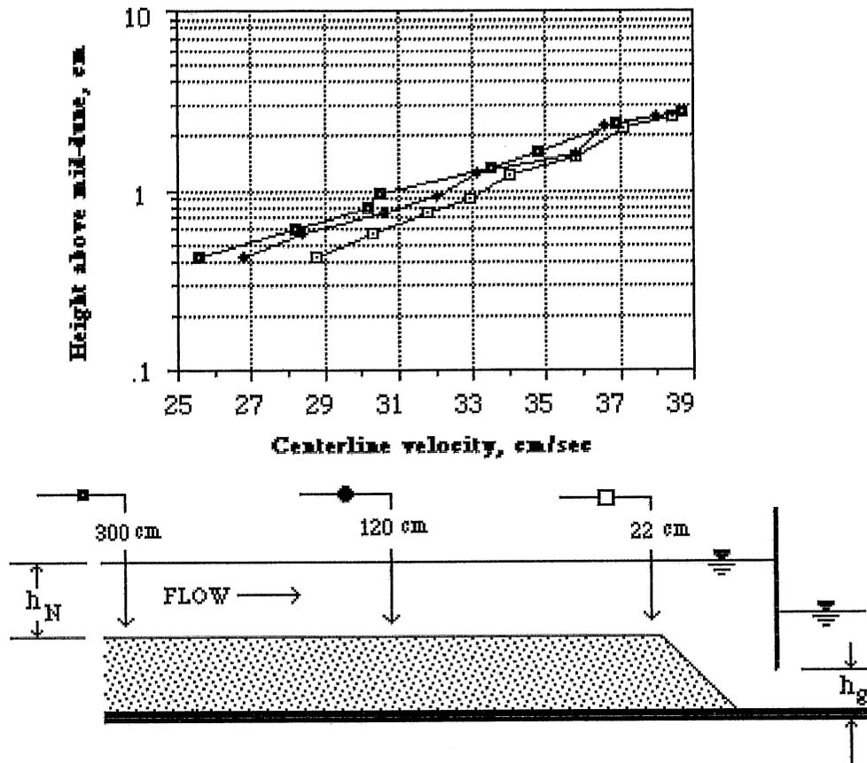
**Figure A2.4 Centerline velocity profiles for Run 11**
