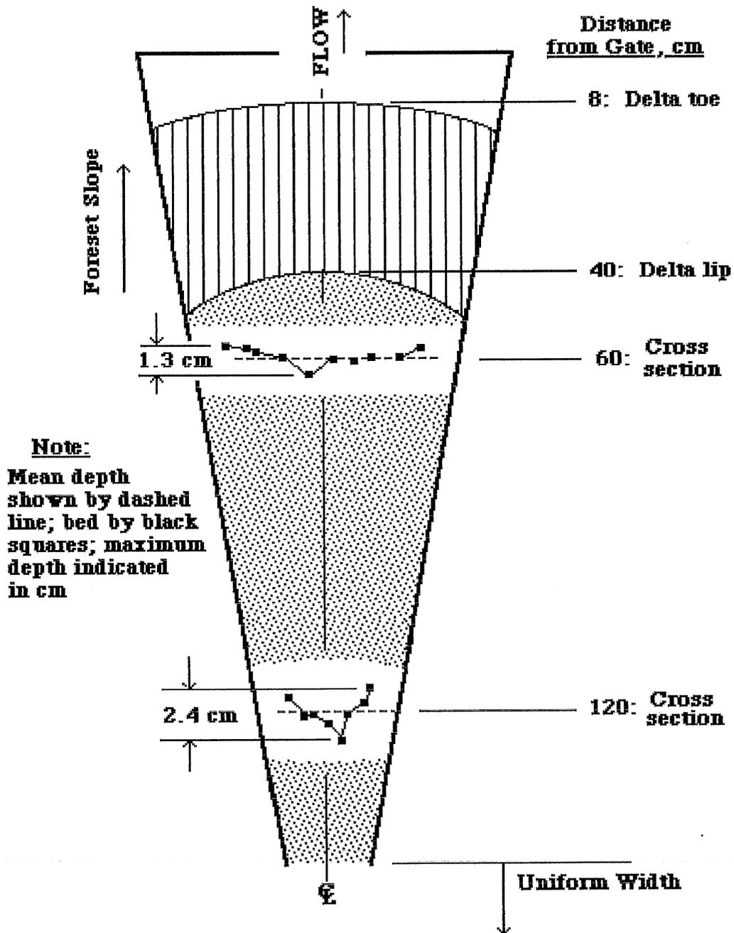
Figure A2.10 Plan view of expanding region upstream of dam for Run 19
