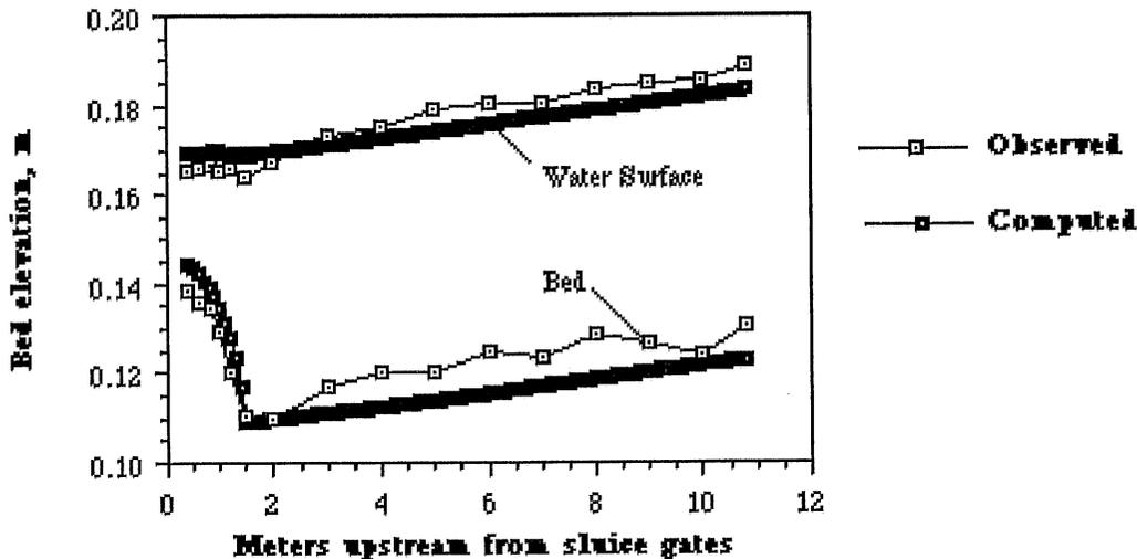
**Figure 4.13 Observed and computed final equilibrium profiles for Run 29**
