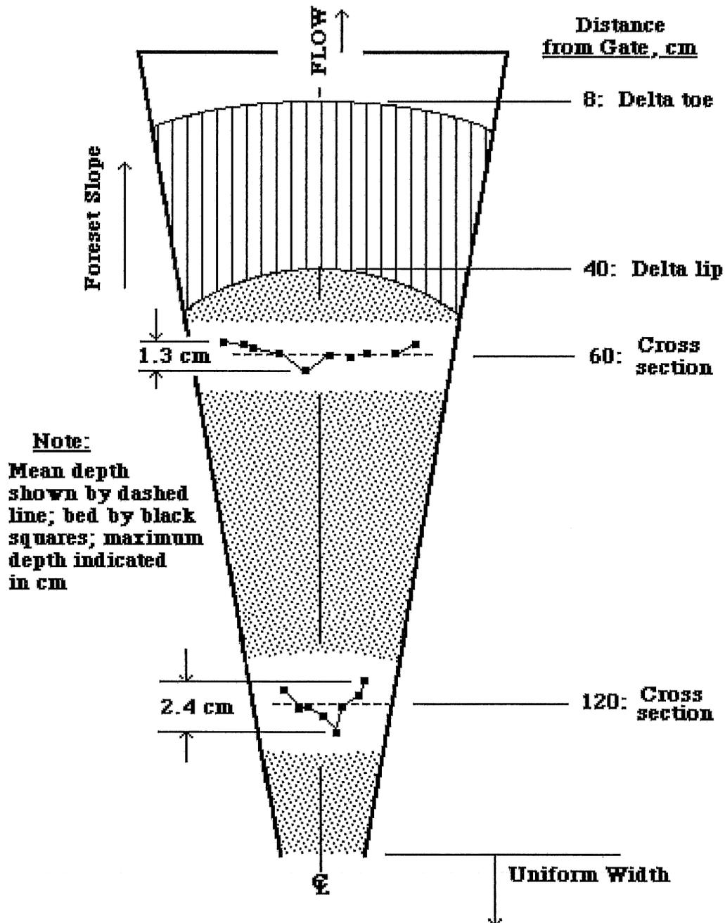
Figure 3.6 Plan view of expanding region upstream of dam for Run 19
