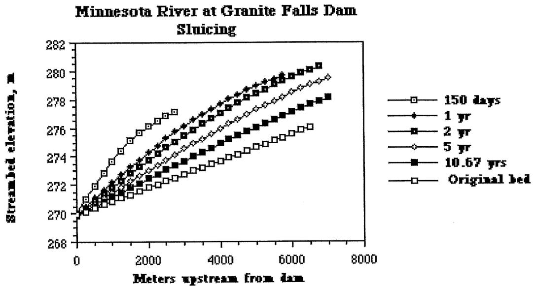
**Figure 4.17** Computed bed profiles for the remainder of the sediment sluicing simulation period
