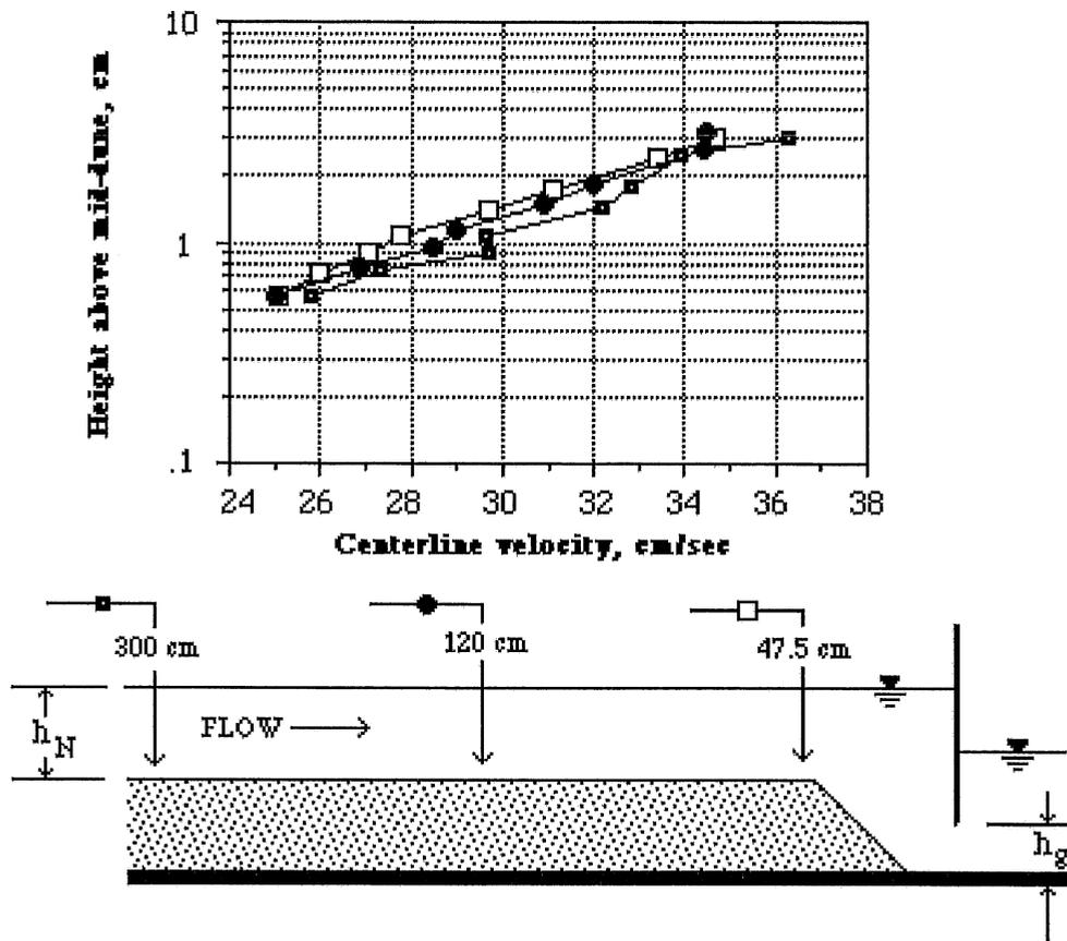
**Figure 3.6 Centerline velocity profiles for Run 5**
