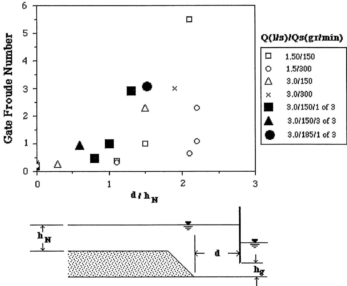
**Figure 3.13 Dimensionless distance upstream of sluice gate(s) for which the flume bottom was exposed**
