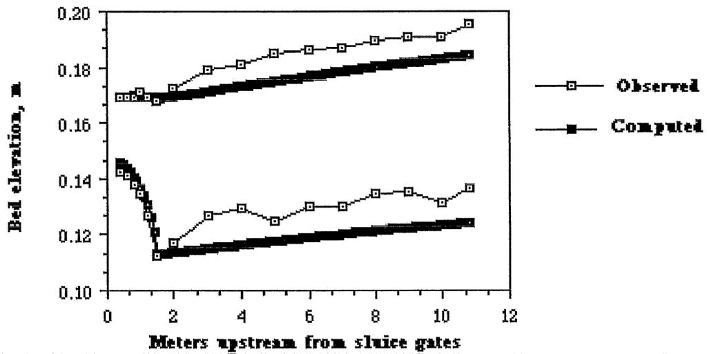
**Figure 4.12** Observed and computed profiles 8 hours later for Run 29
