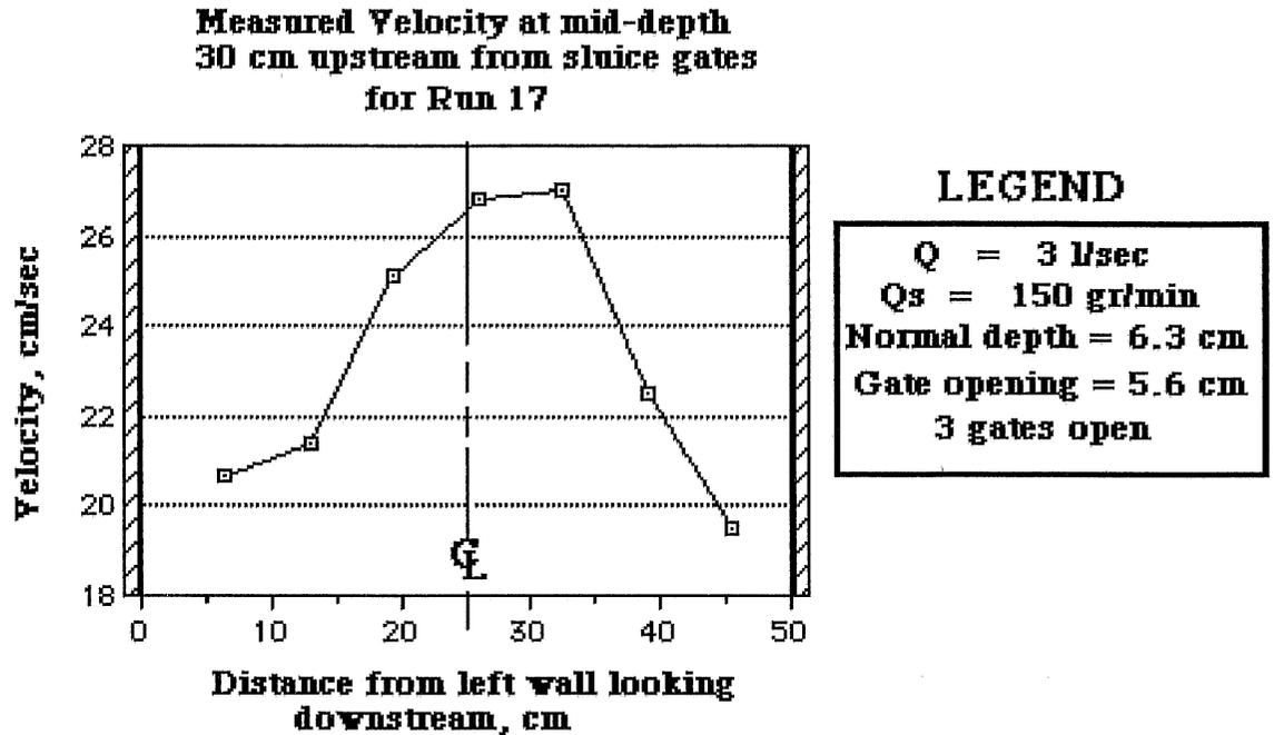
**Figure 3.10 Mean velocity at one-half depth at a location 30 cm upstream from sluice gates in diverging flume for Run 17**
