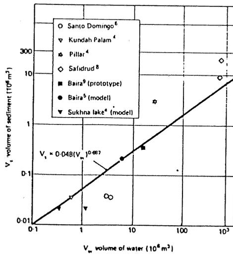
Figure 2.2 Variation of sediment flushed with water used (from Paul and Dhillon, 1988)
