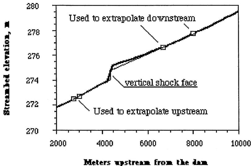
Figure 4.1 Establishing the height of the vertical shock face
