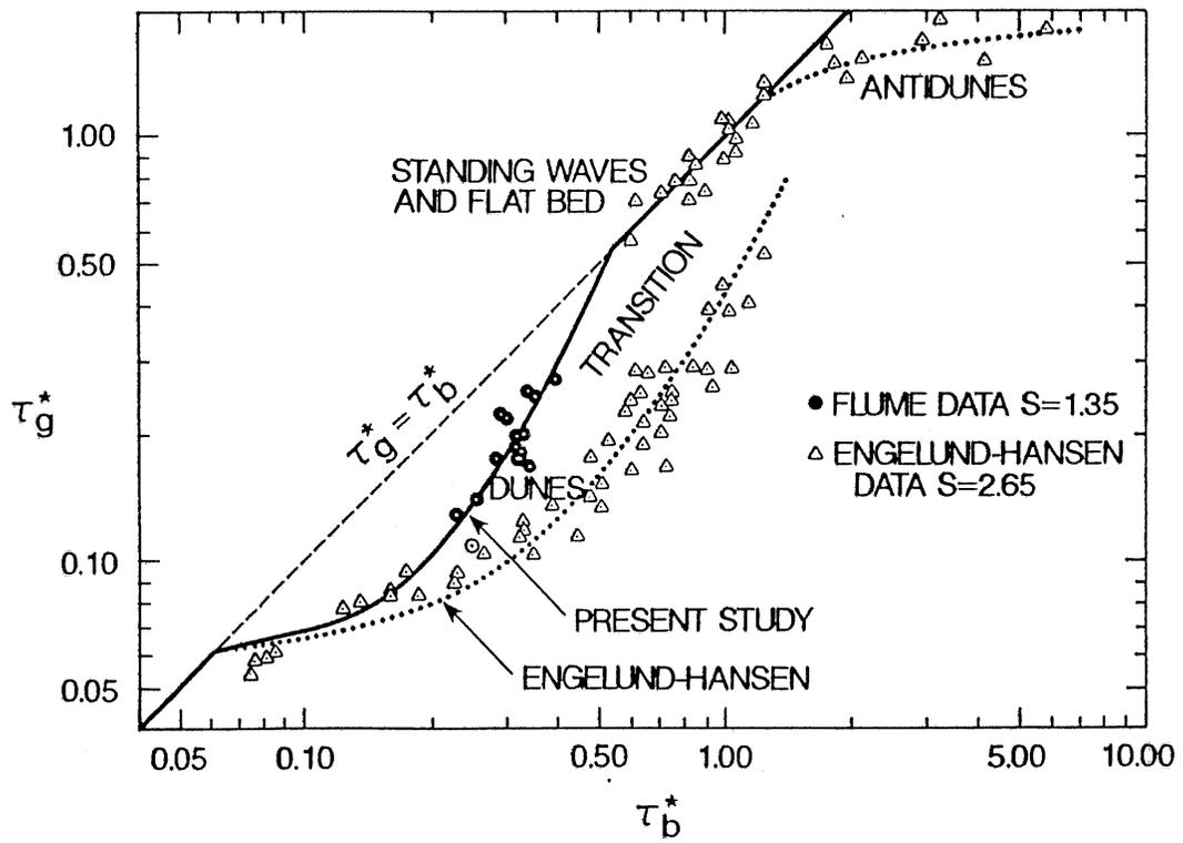
Figure 3.12 Dimensionless grain shear stress versus dimensionless bed shear stress
