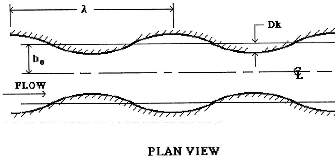
**Figure 5.3 Uniform rectangular channel with a sinusoidal perturbation in width**
