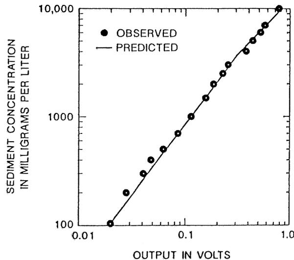
Figure 3.5 Calibration of electro-optical concentration meter
