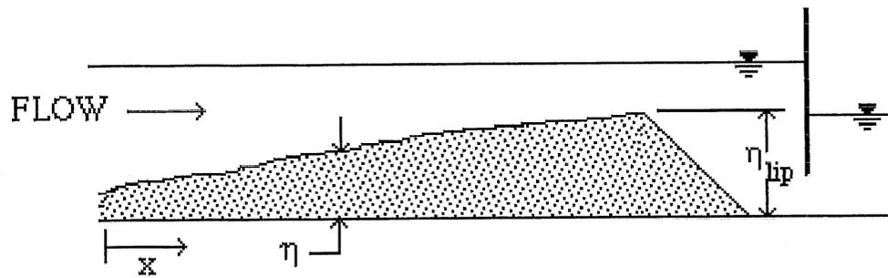
**Figure A2.13 Dimensionless longitudinal bed profile in expanding region upstream of dam for Run 18**
