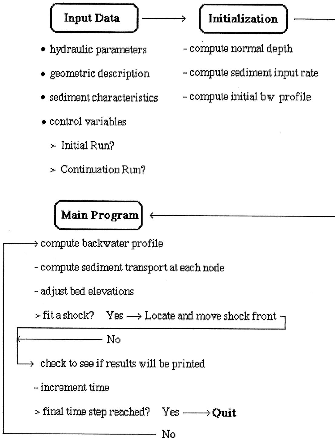
**Figure 4.3 Flowchart for numerical model of reservoir aggradation and degradation**
