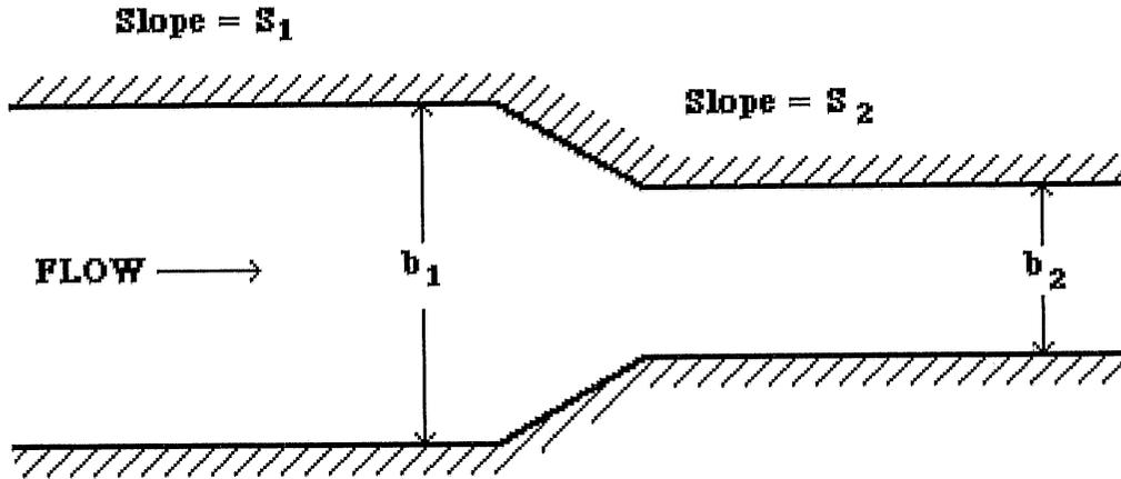
**Figure 5.1 Plan view of channel with long contraction**
