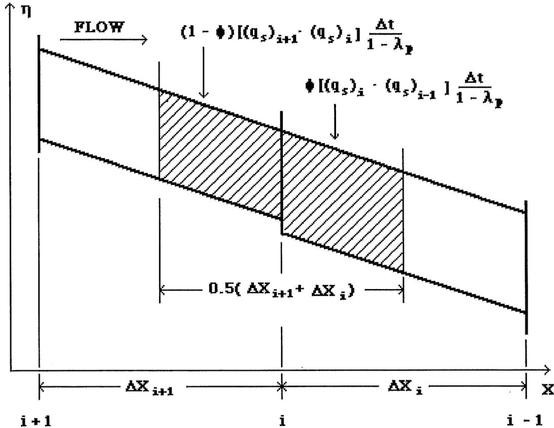
**Figure 2.4 Schematic diagram for explicit finite difference scheme**
