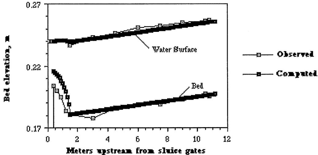
**Figure 4.7 Observed and computed final equilibrium profiles for Run 28**
