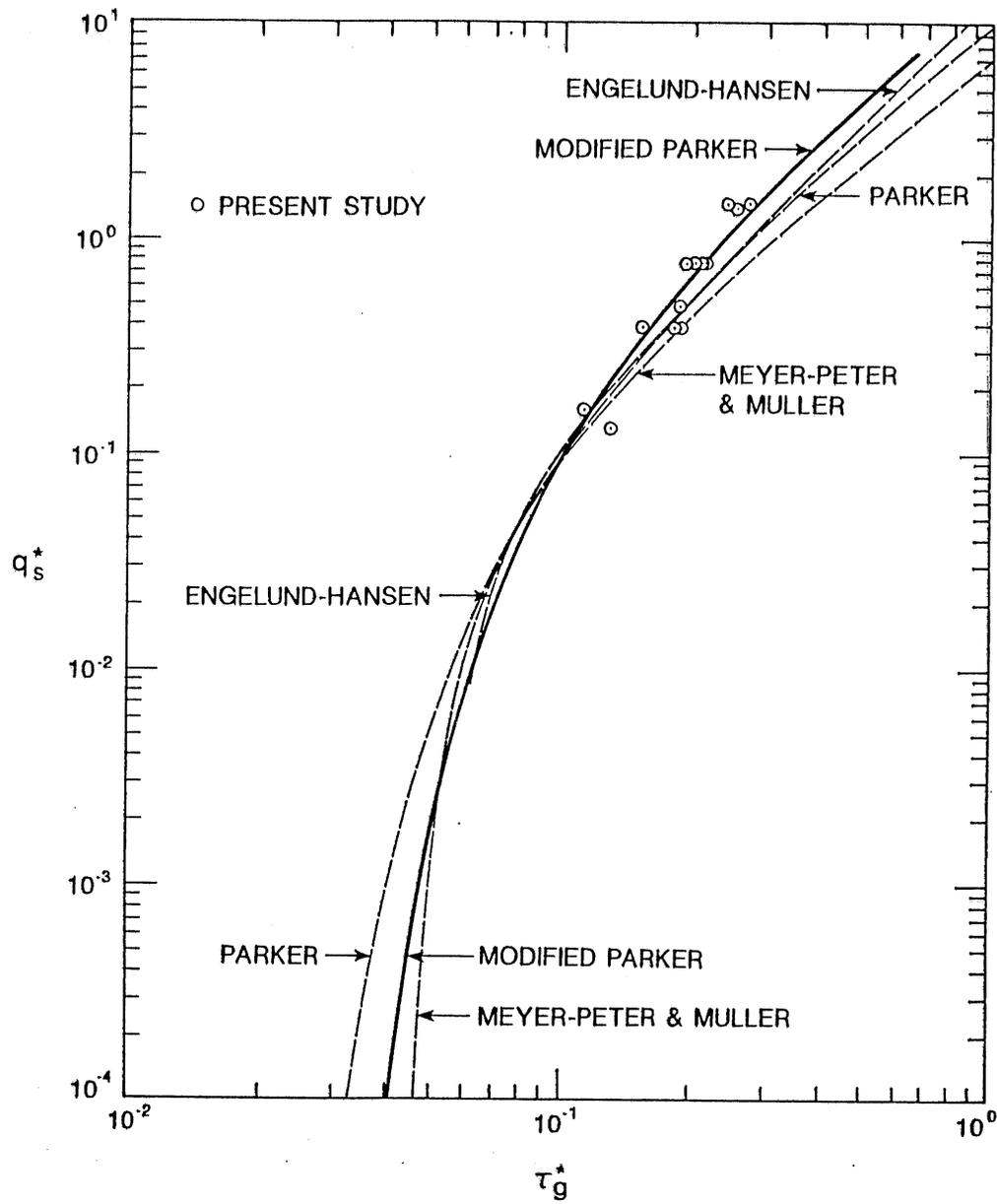
**Figure 3.11 Dimensionless sediment transport per unit width versus dimensionless grain shear stress**
