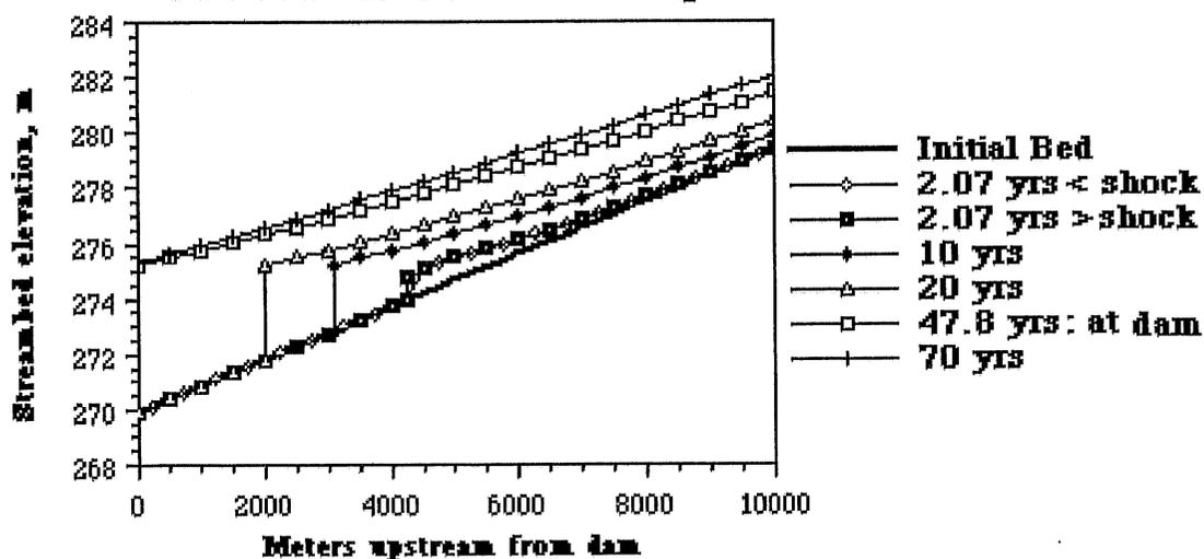
**Figure 4.15 Computed bed profiles for field case with length of backwater zone 5 times initial length**
