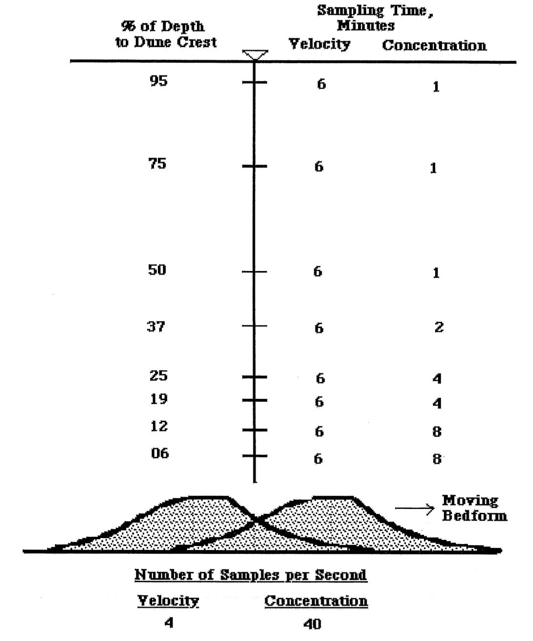
**Figure 3.4 Velocity and sediment concentration sampling intervals, frequencies, and locations**
