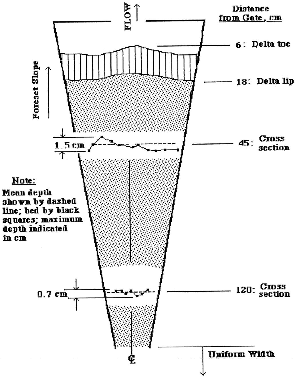
Figure A2.9 Plan view of expanding region upstream of dam for Run 18
