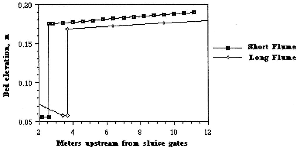
**Figure 4.9 Computed bed profiles when the delta is about 3 meters upstream of the sluice gates for the 12-meter-long and 120-meter-long backwater reaches**
