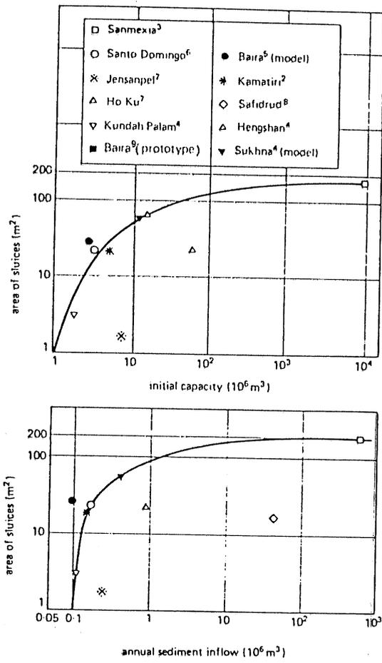
Figure 2.1 Suggested design curves for flushing sluices (from Paul and Dhillon, 1988)
