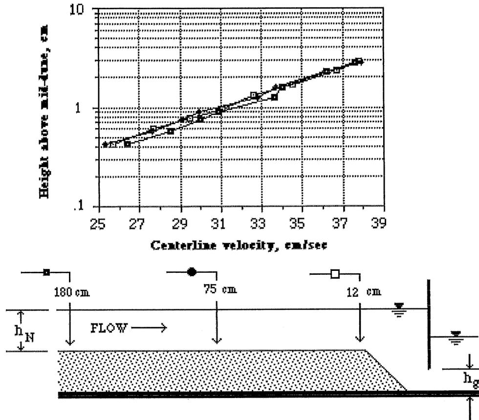
**Figure A2.3 Centerline velocity profiles for Run 7**
