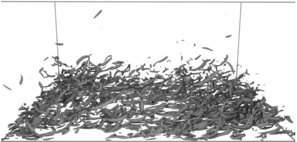
Figure 3.2: An entire view of vortices in a turbulent channel flow identified by iso-surface extraction on swirl strength.
