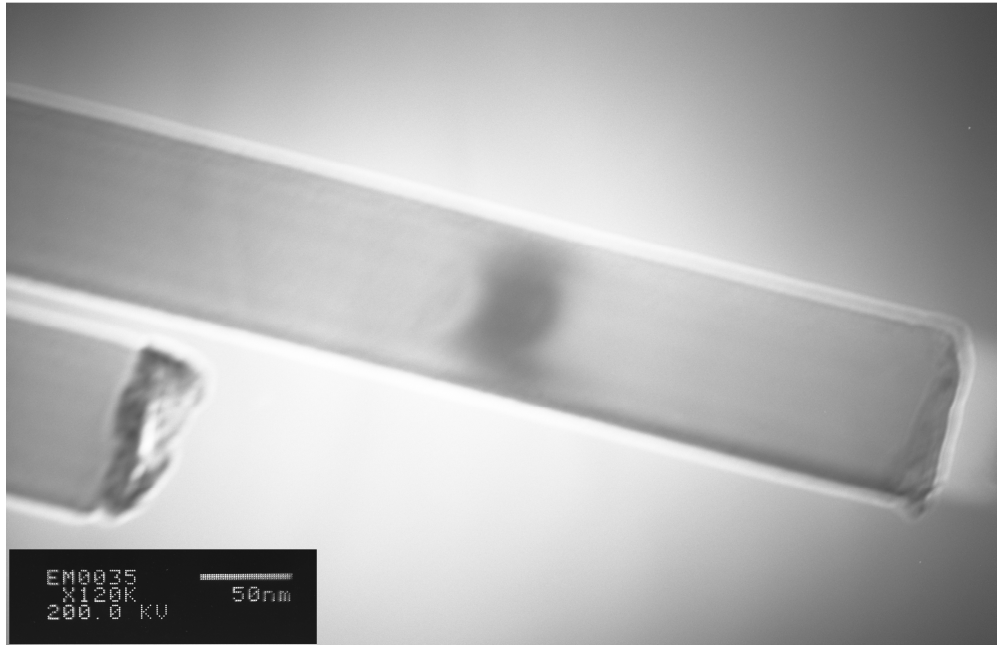
Figure 4.18. Bright field image of 100 nm pillar in 200keV microscope. Strain field is broad, as seen in figures 4.14 and 4.16. Micrograph courtesy of Dr. Ozan Ugurlu.
