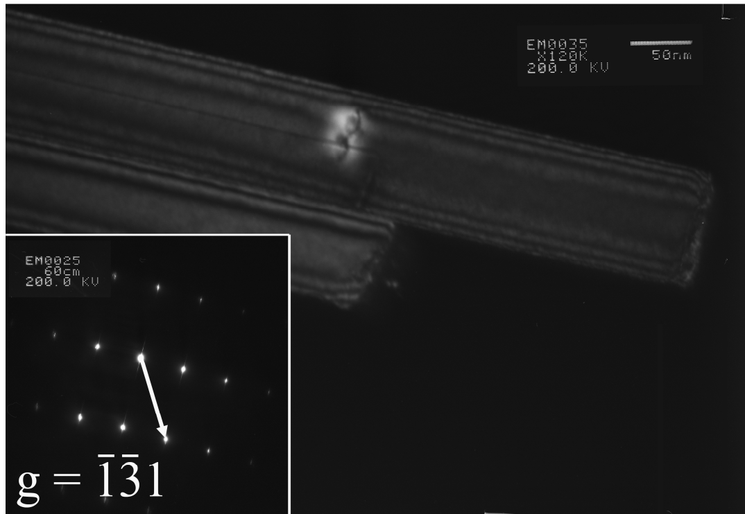
Figure 4.19. Dark field image of the singly compressed 120 nm diameter pillar, with clear indications of a dislocation strain field, which relaxes at the surface. Courtesy Dr. Ozan Ugurlu.
