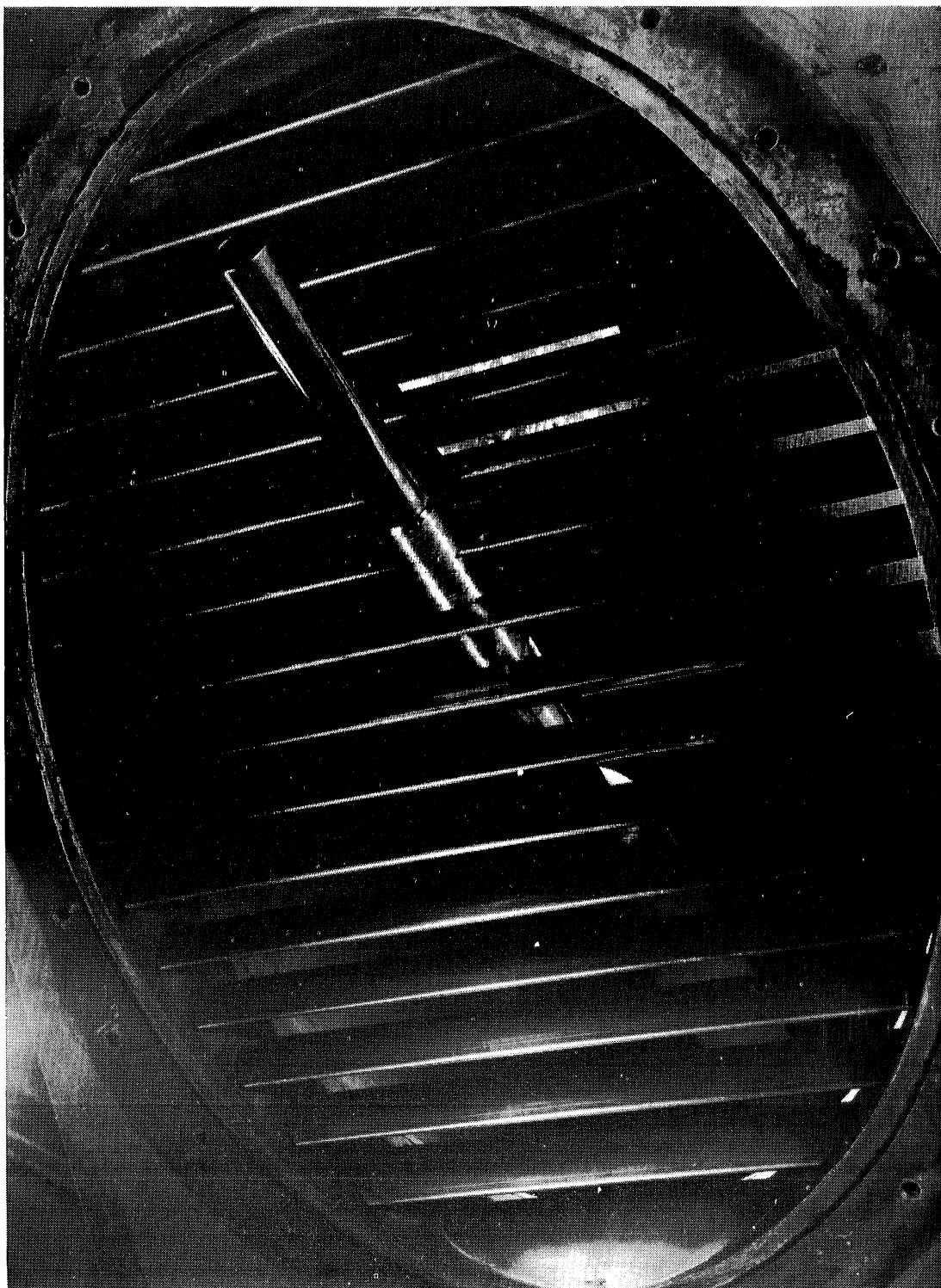
Fig. 7 - Intersection of Contraction Dynamometer Shaft with Vaned Elbow IV (Tunnel Form B)
