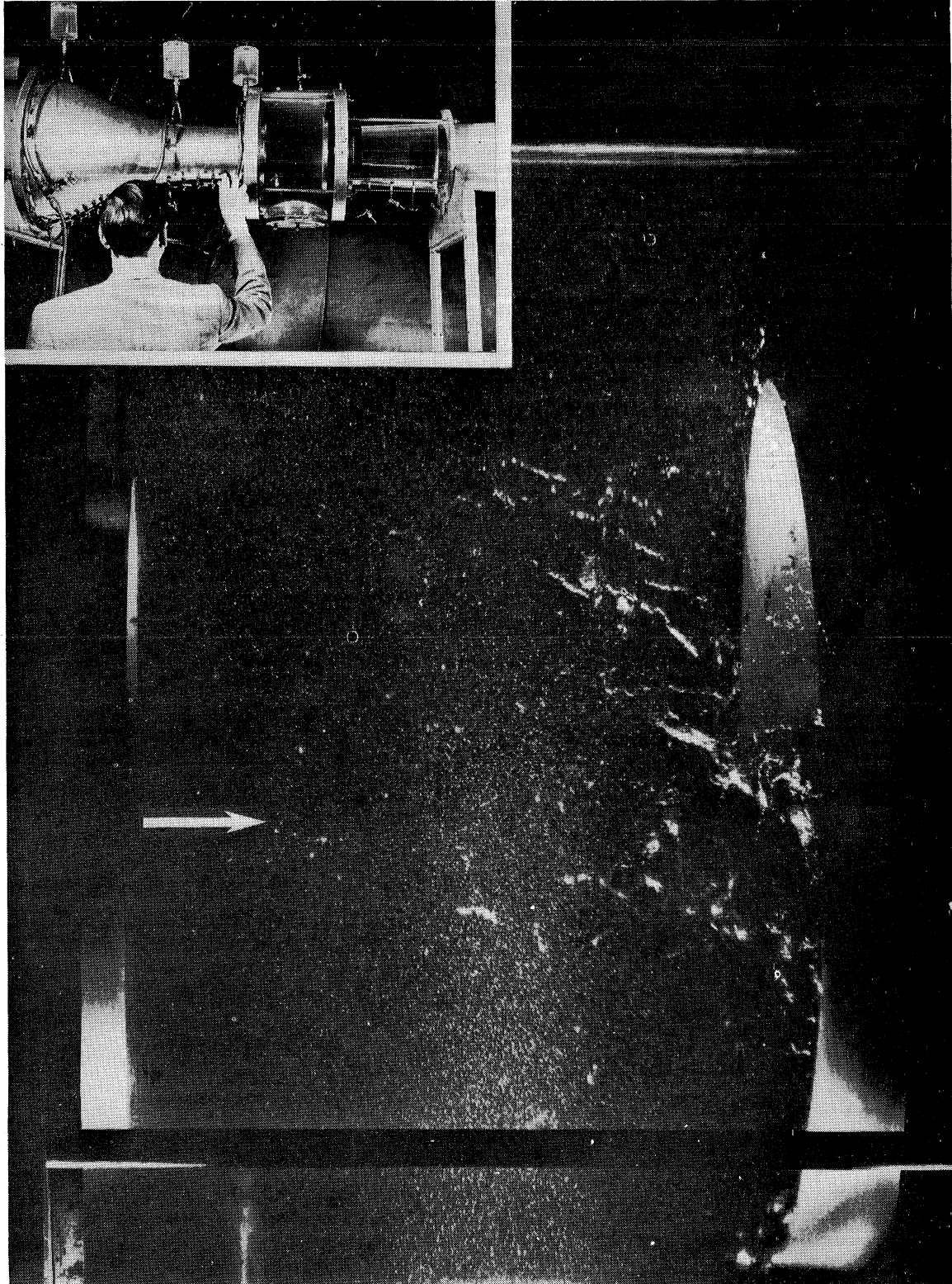
Fig. 39 - Severe Cavitation in the Diffusion Layer of the Model Open-Jet Test Section
