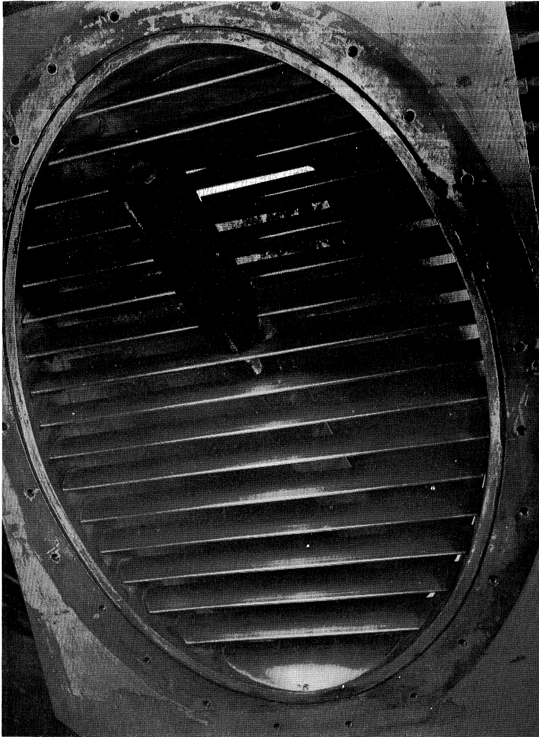
Fig. 8 - Intersection of Contraction Dynamometer Shaft with Vaned Elbow IV (Tunnel Form H)
