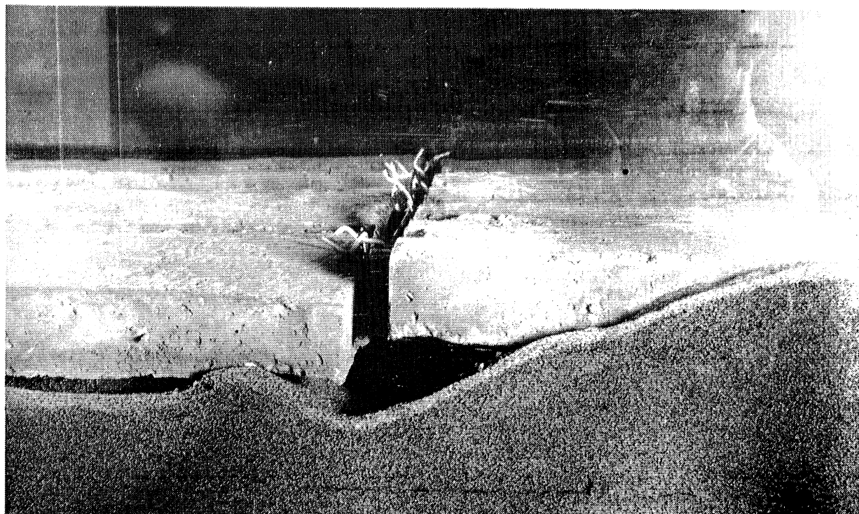
Fig. 18 — Effect of Step-up on Sand Scour
