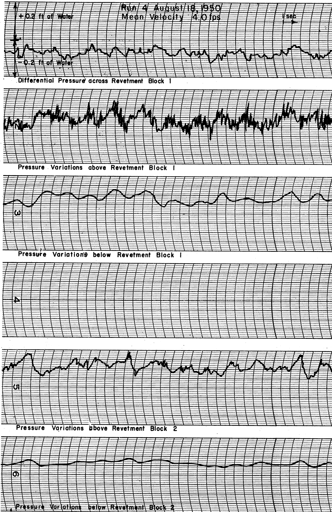
Fig. 30— Sample Pressure Fluctuation Record
