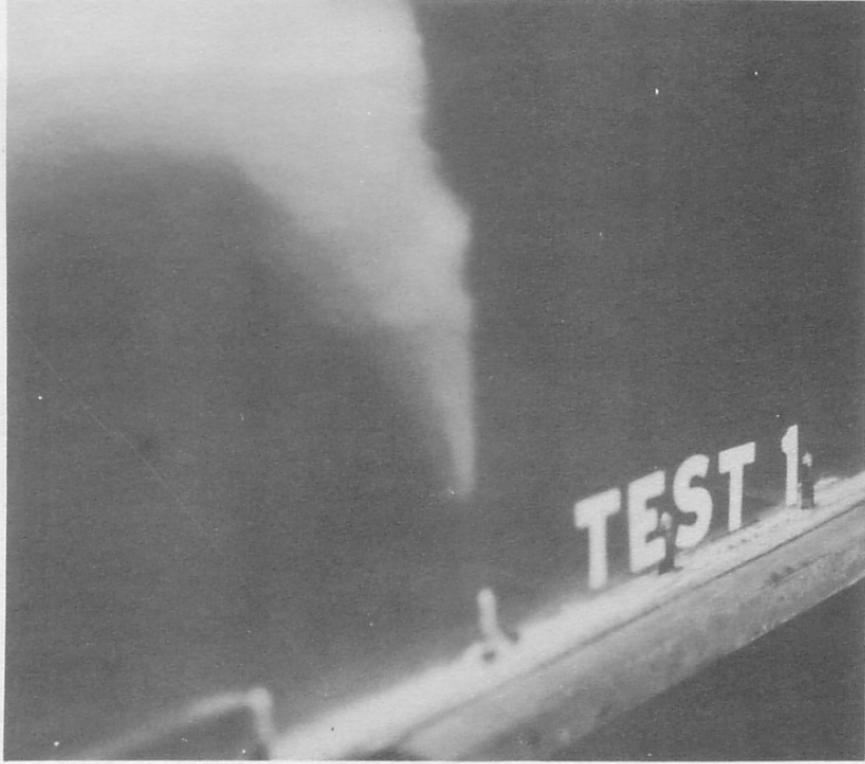
a. - Typical Air-Water Mixture Jet
