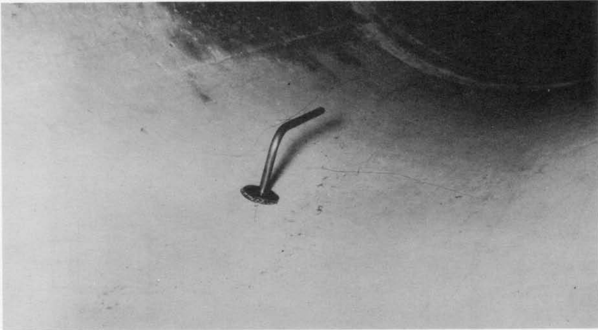
Fig. D-2 - View of Static Tubes Installed in the 36-in. Cast Pipe
