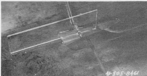
(e) H/D = 1.01 . Just after inlet has sealed. There is no air entering.
