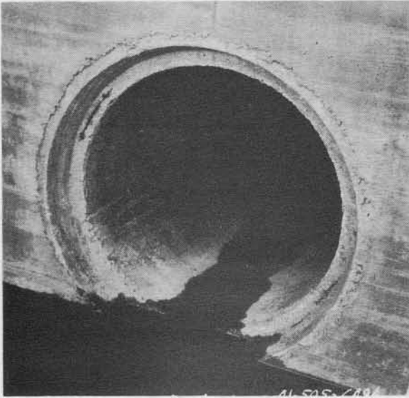
Fig. IX-3 - Concrete Pipe Groove Entrances, Experiment 1, Stillwater, Oklahoma.
