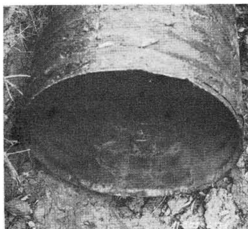
Fig. IX-9 - Cracking of Bituminous Coating of 24-in. Corrugated Metal Pipe, Stillwater, Oklahoma. n = 0.0218 .
